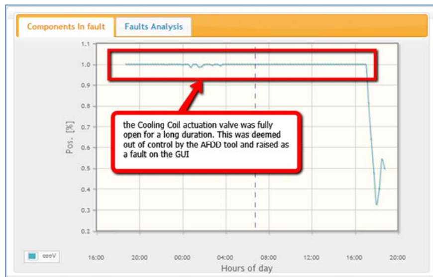
Figure 6: Site 1 AFDD tool repair effectiveness check (2)
