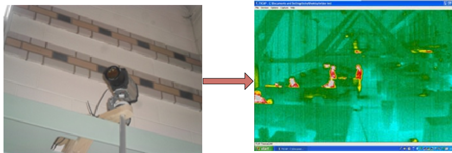
Figure 3. Ground truth occupancy data using infrared camera
