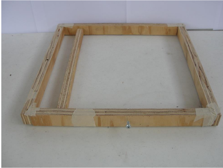
Figure 56: Single bar passive resistive piece for the 2 ton unit.
