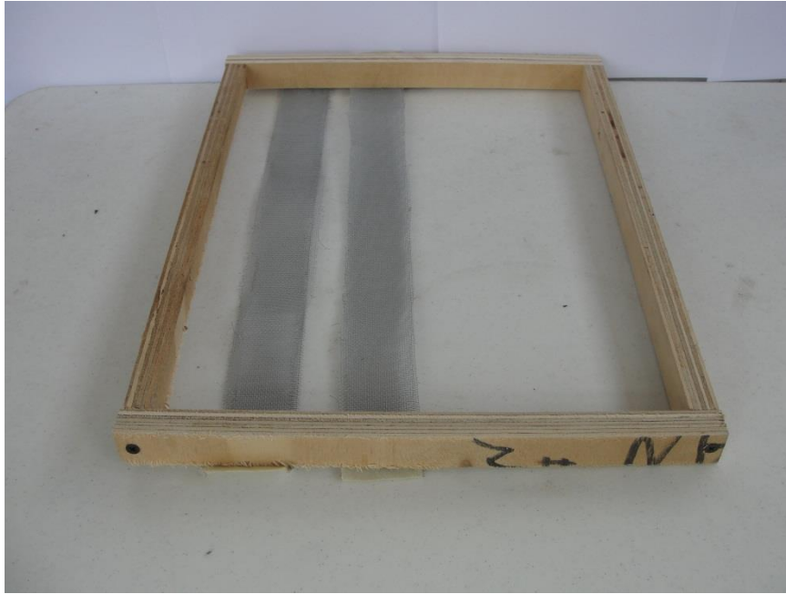
Figure 61: Double strip mesh for the 3 ton unit.
