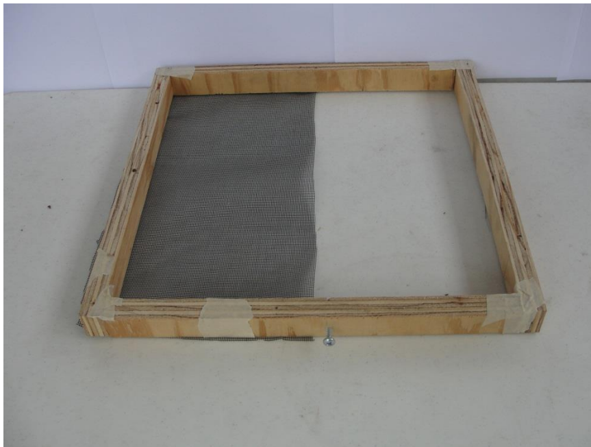
Figure 55: Half plastic mesh passive resistive piece for the 2 ton unit.
