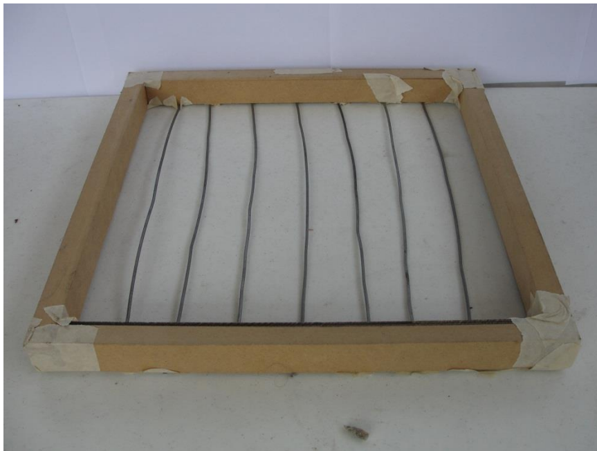
Figure 57: Parallel rods passive resistive piece for the 2 ton unit.
