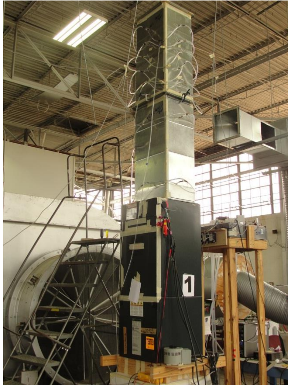
Figure 40: ASHRAE Standard 37 static pressure measurement verification.
