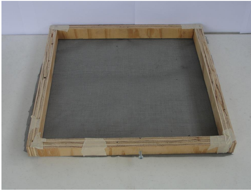
Figure 54: Plastic mesh passive resistive piece for the 2 ton unit.
