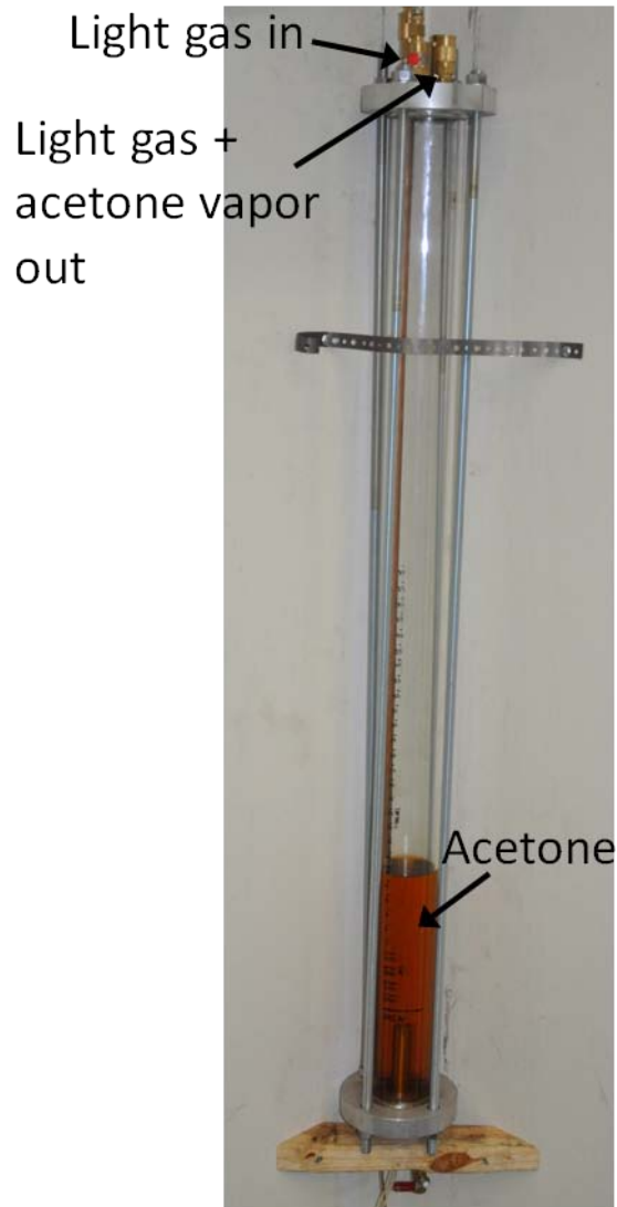
Figure B.5: Acetone bubbler.
