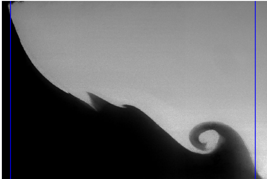
Figure 4.18: Sample Mie scattering image processed to find the 5% and 95% contours shown by the blue lines at 3.38ms.
