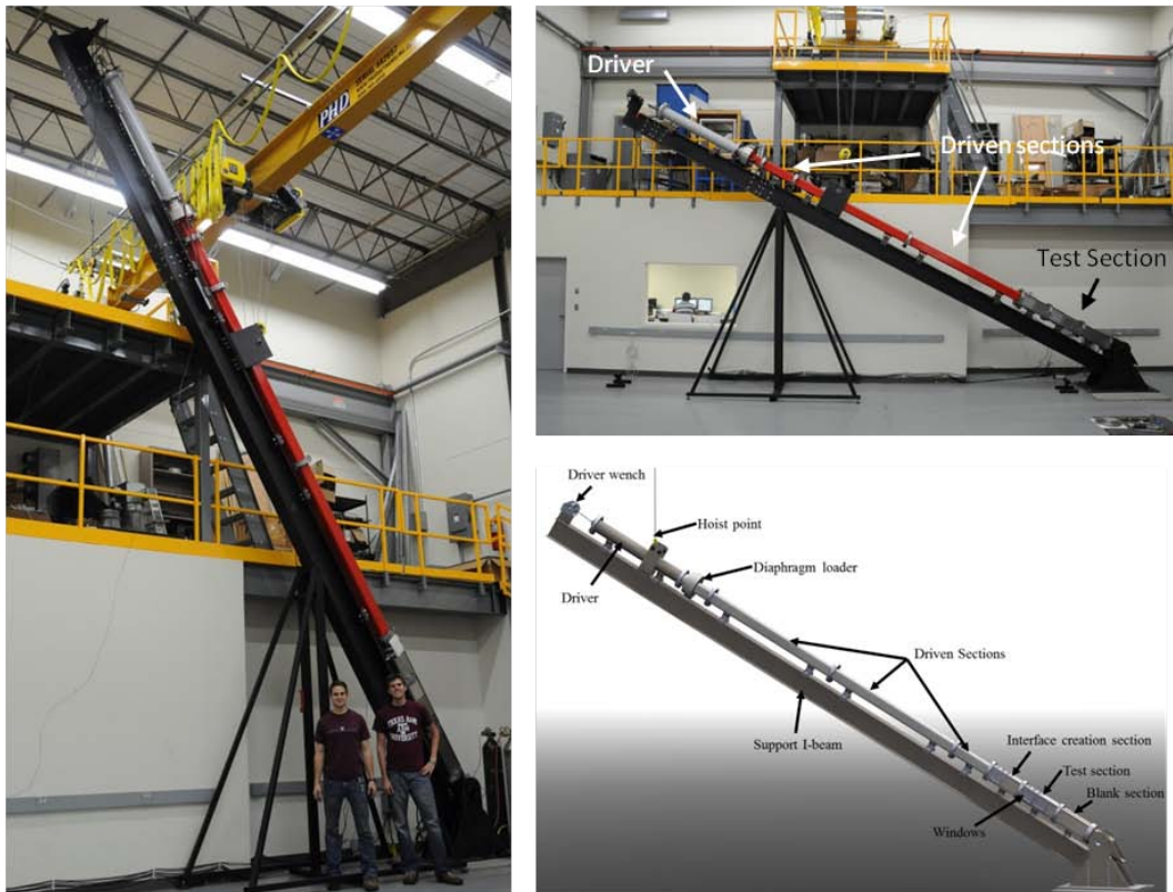
Figure 4.1: The Texas A&M Shock tube facility. Left: the shock tube inclined at 60 degrees, Top Right: the shock tube at approximately 30 degrees inclination, Bottom Right: Schematic of the shock tube with sections labeled. In the Picture: Mr. Chris McDonald and Mr. David Reilly (undergraduate students).
