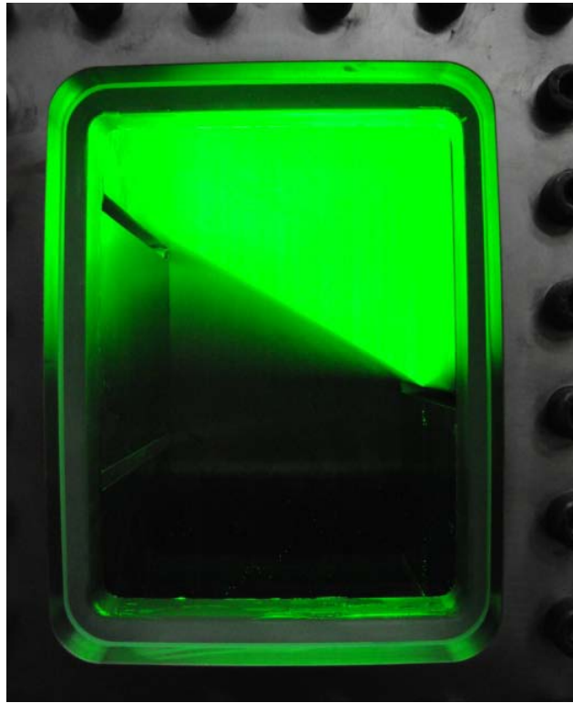
Figure 4.4: Mie scattering signal from a fogged interface using the PIV laser system.
