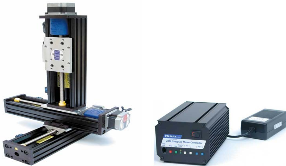
Fig. C-1: (a) Velmex bi-slide for X-Y-Z axes movements (65) & (b) Velmex VXM2 stepping motor controller (66)
