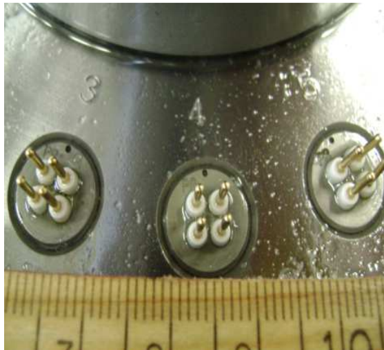
Figure 11: Electrical ports where the pore pressure transducer is connected.
