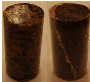
Figure 51: Westerly Granite specimen before and after multistage test.
