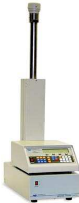
Figure 7: Syringe pump used to reduce the external fluid volume.
