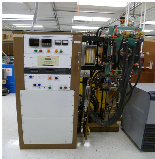
(a) High temperature furnace used for casting the alloys
