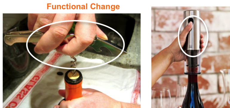
Figure 19. Automating a wine opener eliminates the need for twisting the hand [92]. Typical wine opener is shown on the left and the automatic wine opener is shown on right
