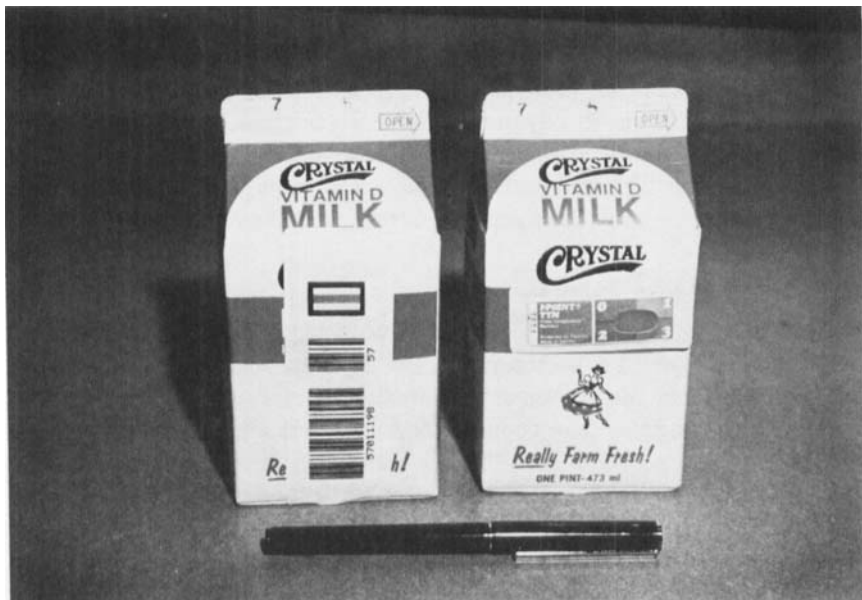
FIG. 1. LIFELINE FRESHNESS MONITOR MODEL 57 (LEFT) AND 1-POINT TIME/TEMPERATURE MONITOR MODEL 2140 (RIGHT) PLACED ON 1-PINT CARTONS OF PASTEURIZED MILK
