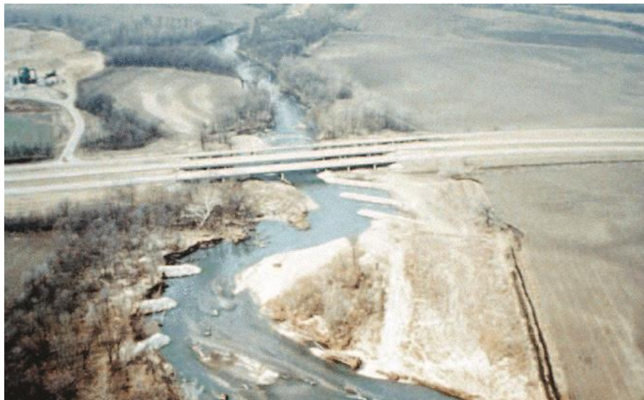
Figure 6-17. Use of Spurs to Redirect Stream Flow (Ryan et al. 2006).
