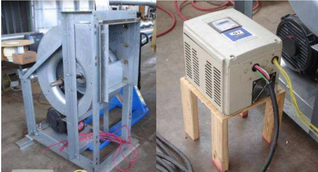
Figure 3: Blower (left) and VFD (right)
