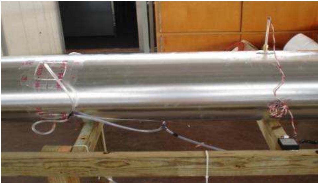
Figure 5: Piezometer Ring (left) and Temperature Sensor (right) Mounted
