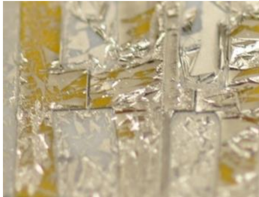
Figure 16: Delaminated Nickel film on Al 2 O 3 substrate
