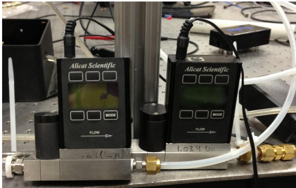
Figure 5: Alicat flow meter regulating gas flow rate and gas mixture ratios flow rate values are 10.24 SLPM and 1.024 SLPM
