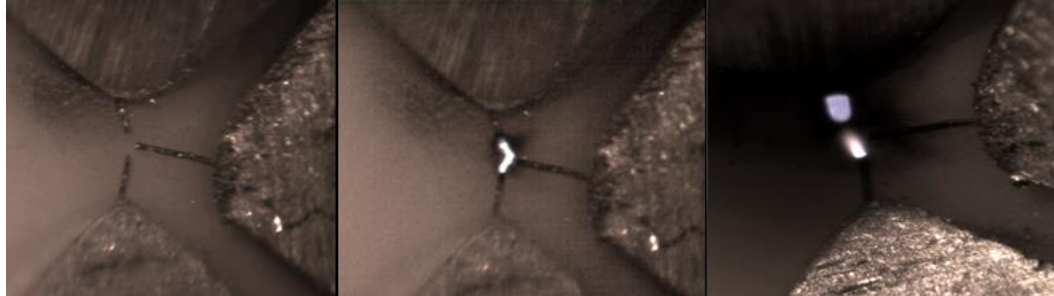
Figure 26: 3-Electrode gated configuration using 50 \mu\text{m} Pt-13%Rh alloy wire before (left), during (middle) and post switching (right)
