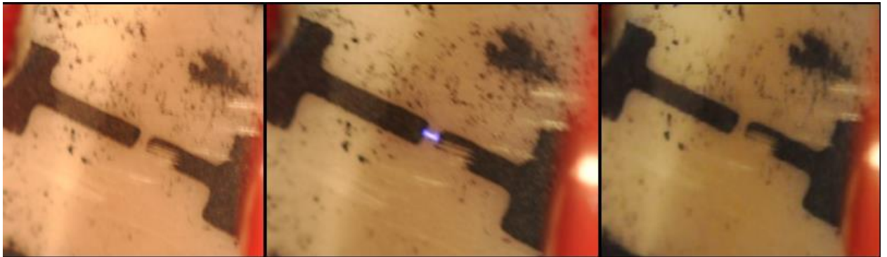
Figure 30: Titanium Titanium-Oxide on CSZ before, during and after discharge 800 nm thick layer with 150um gap, 0.75 mA and 2.6 kV coating oxidized during photoresist removal
