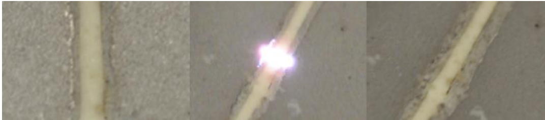
Figure 27: Nickel on CSZ substrate before, during and after 120 nm thick layer 250 \mu\text{m} gap pre-test and \sim 500 \mu\text{m} gap post-test
