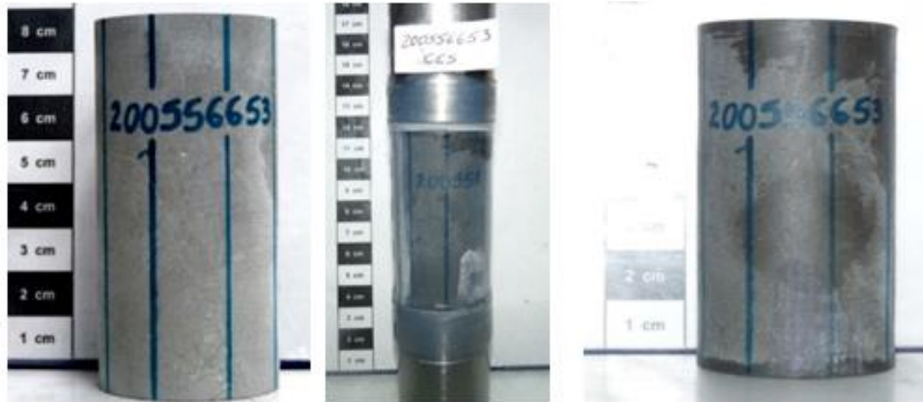
Fig. 5.16—San Antonio cement sample, after a triaxial test with confining pressure of 12,000 psi
