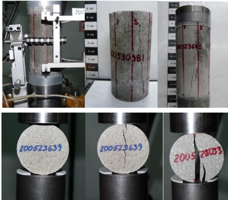
Fig. 5.10—Photos of uniaxial and tensile strength tests for 15.6-ppg FlexStone cements
