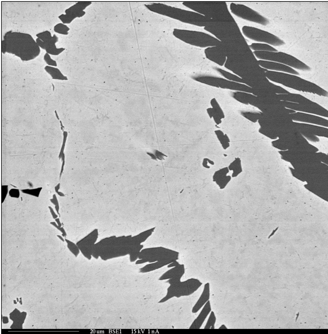
(b) Zirconium dendrites within \delta -UZr 2 matrix phase in U-50ZrAC (1000X)
