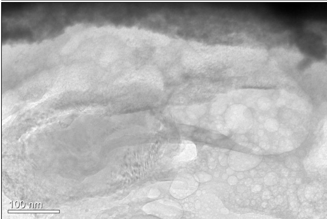
Figure 4-37: Moving and coalescing bubbles found from U-0.1ZrAl5.
