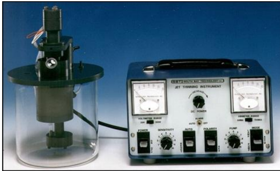
(a) Apparatus of the electropolisher (figure courtesy of South Bay Technology)
