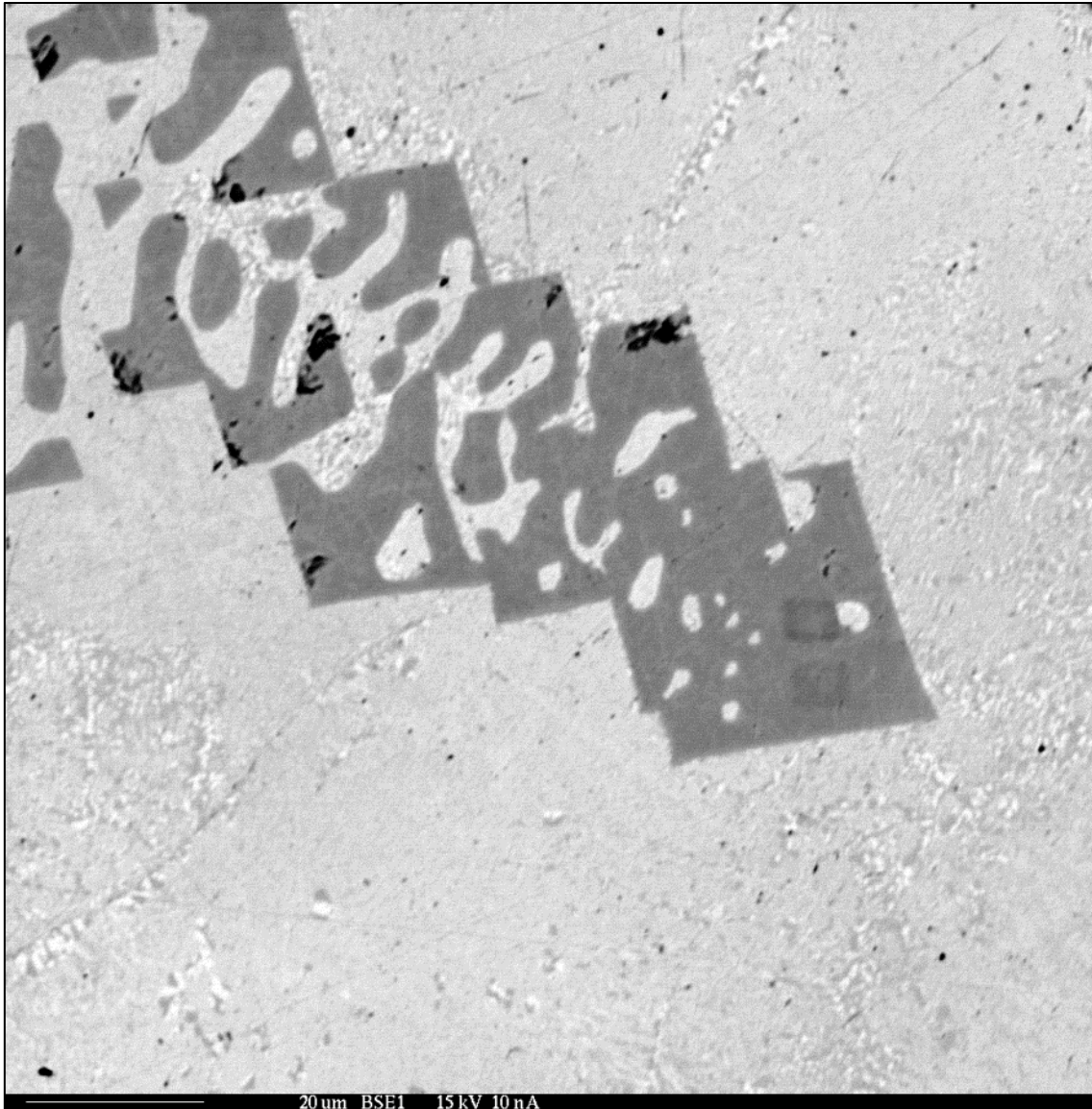
Uranium mononitride (UN) particles in U-10Mo28d500 (750X)
