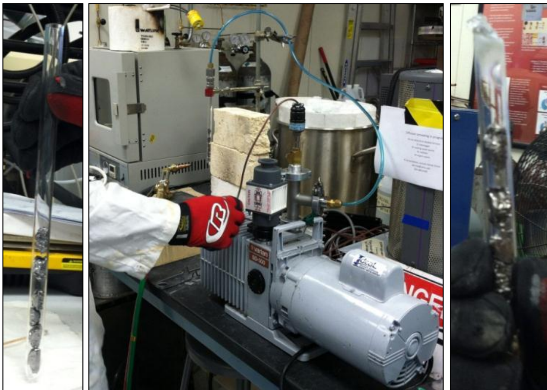
Figure 3-2: Tantalum foil wrapped U-Zr alloy buttons sealed in a quartz tube connected to a roughing pump for further annealing; before (left), during (center), and after (right) the sealing.
