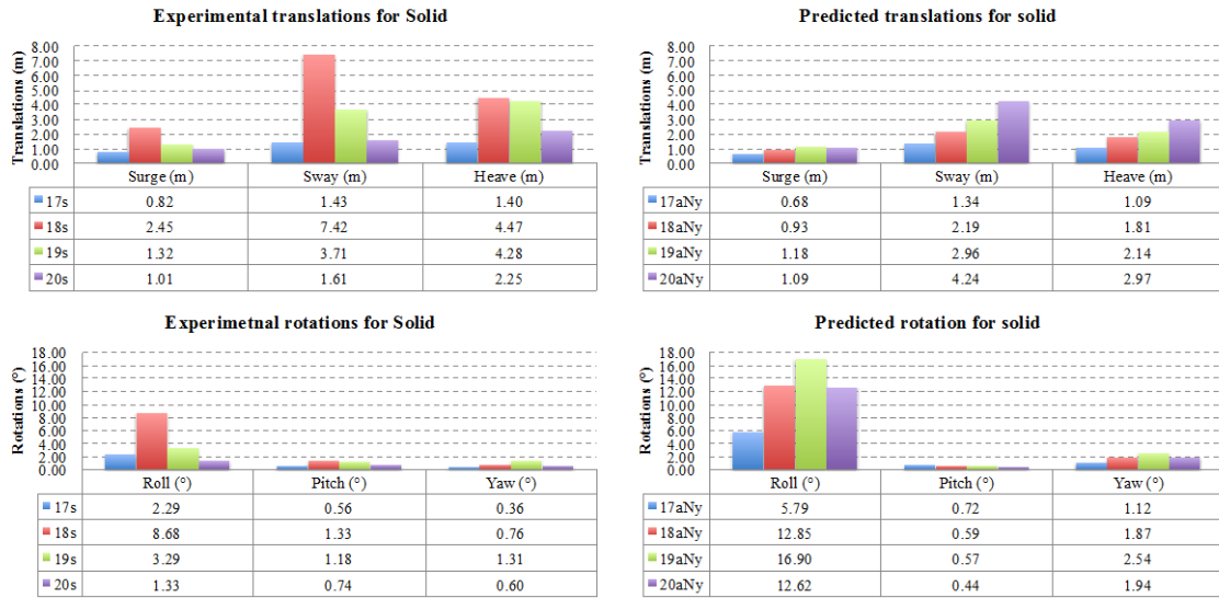
Figure 29. Comparison of the numerical and experimental results of the effect of wave direction on moored ship motions.
