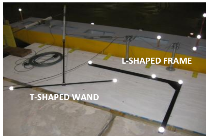
Figure 14. L-shaped bar and wand on the model dock with moored ship prior to calibration
