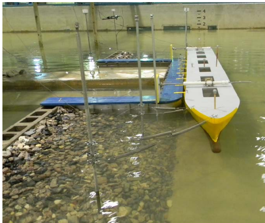
Figure 2. Model container ship moored to solid wall dock (top) and schematic of mooring line locations (bottom).
