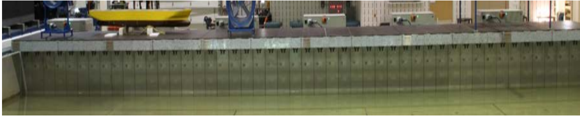
Figure 9. Multidirectional wave generator with 48 individual paddles.
