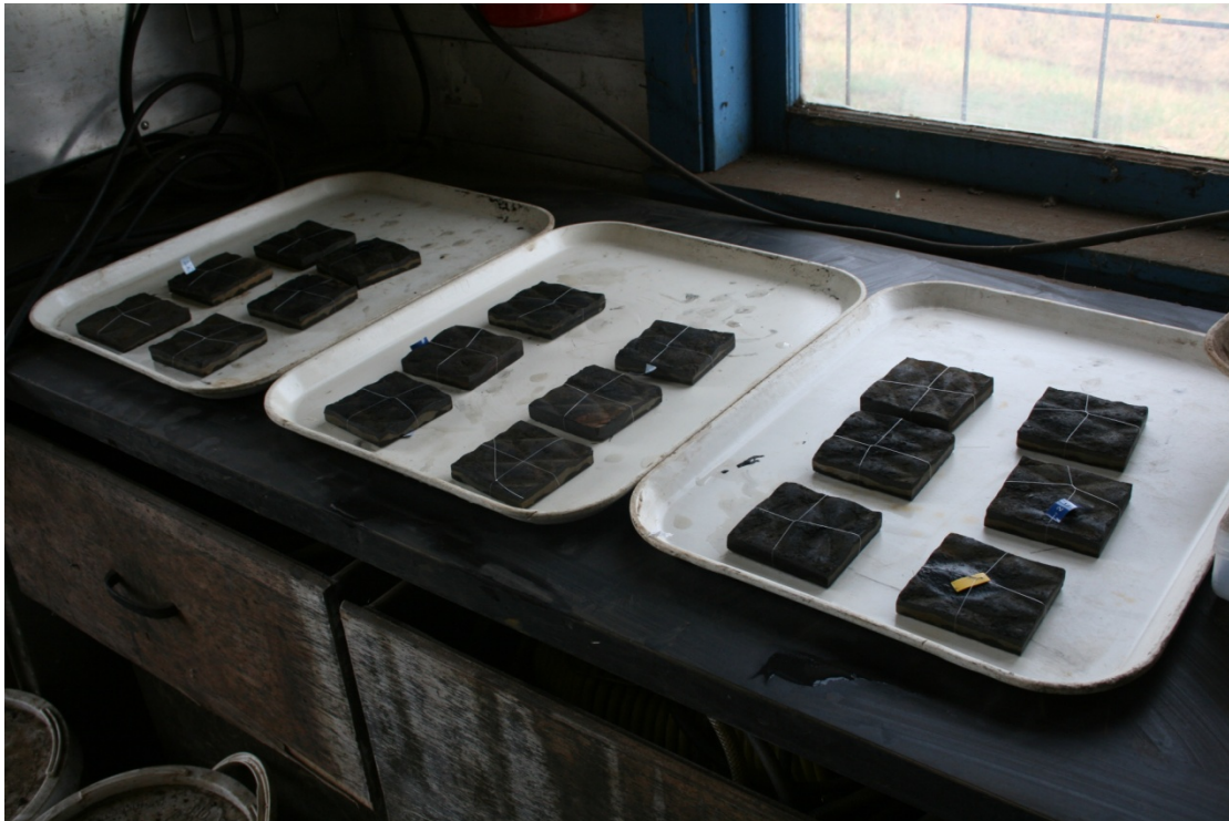
Figure 3.2. Cast iron coupons left to dry after 30 minutes.
