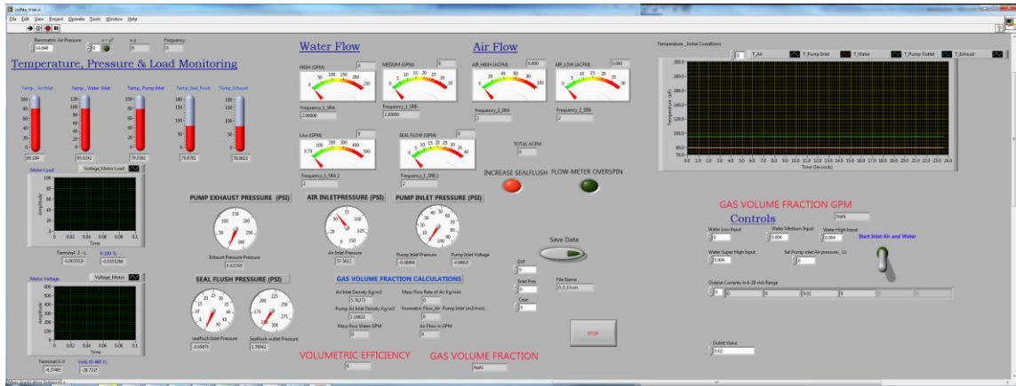
Figure 5.5: LabVIEW front panel for monitoring, recording and controlling the parameters
