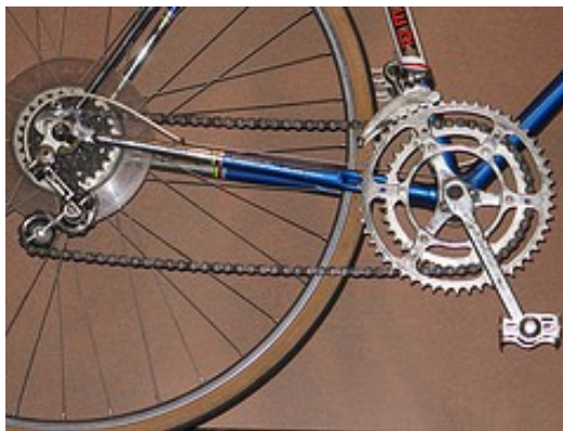
Figure 15: Direct energy transfer from pedals to rear wheel through gears and chain (Flickr, 2010)
