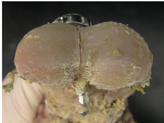
Figure 73. LCP #1 after single ramp to failure experiment. The bone/plate construct failed about the most distal face on the proximal phalanx bone along the holes created by the locking screws and cortical bone screws.
