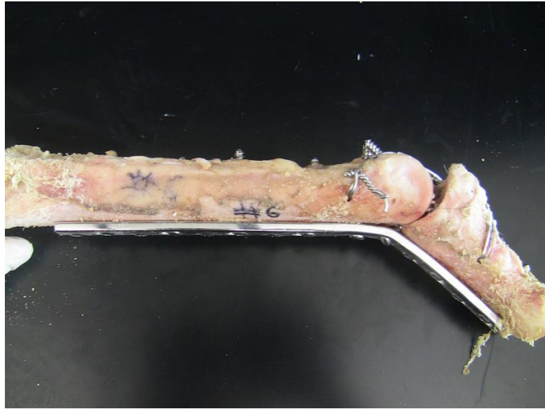
Figure 72. DCP #6 after single ramp to failure experiment. Consistent with the other DCP test specimens, the bone screws and transarticular screws suffered from bone pullout. It is possible that there was bone failure around a cortical bone screw right at the MCP joint, but this will have to be determined by radiograph.
