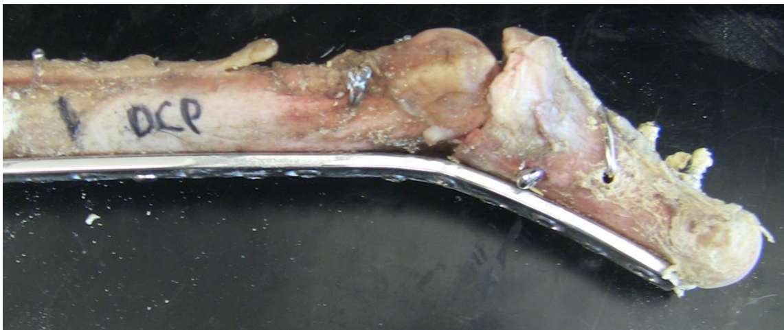
Figure 68. DCP #1 after single ramp to failure test. This image shows the change in angle of the bone plate construct that results from ramp to failure testing.
