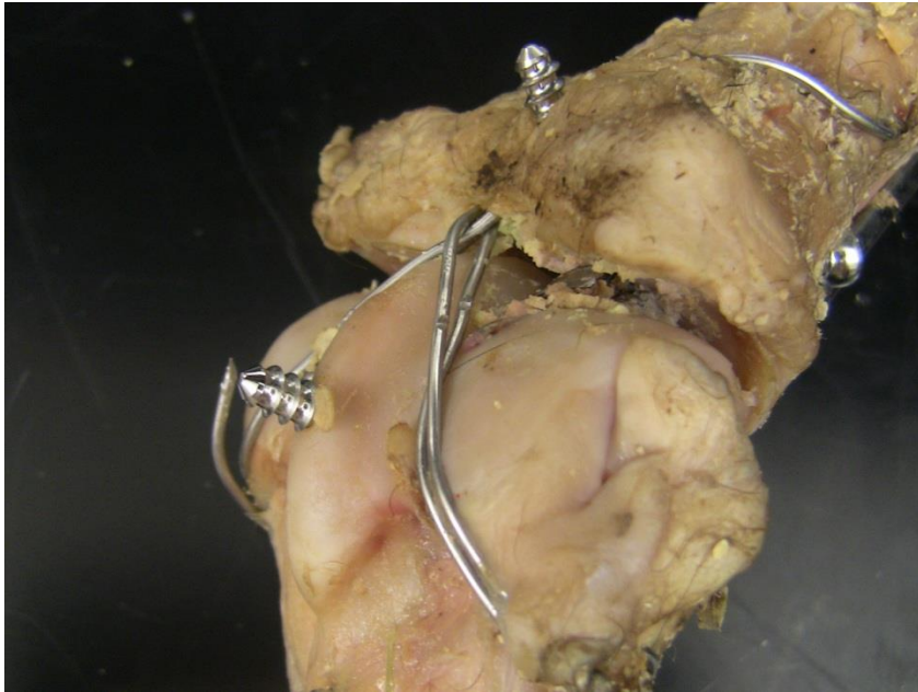
Figure 70. DCP #4 after single ramp to failure experiment. This image shows the failure of the tension band as well as two necking regions. DCP #4 failed by snapping of the tension band as well as pullout of the transarticular screws.
