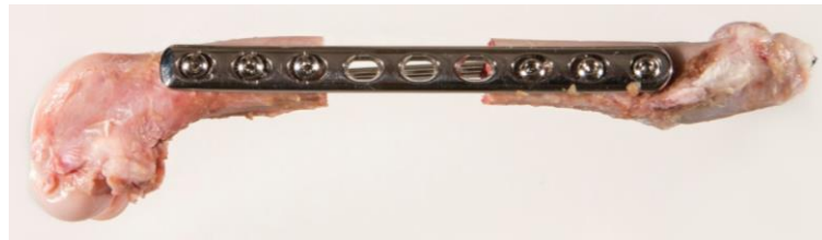
Figure 1. Shown is one of the canine femur test specimens with a simulated comminuted diaphyseal fracture repaired using the LC-DCP and IM pin.
