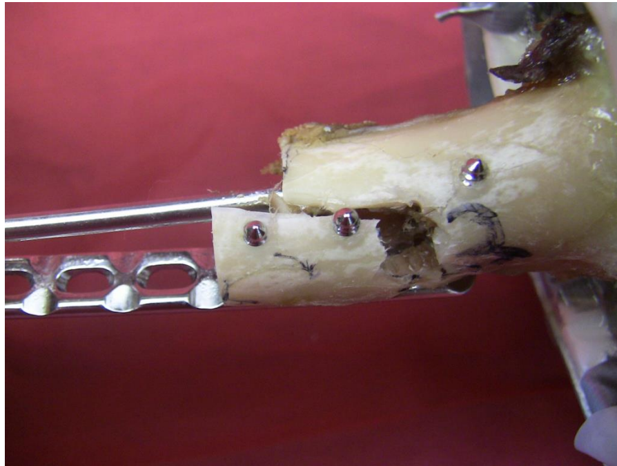
Figure 36. Fracture of LC-DCP #3 from transcortex view. Crack propagates along bone screw – bone interface.
