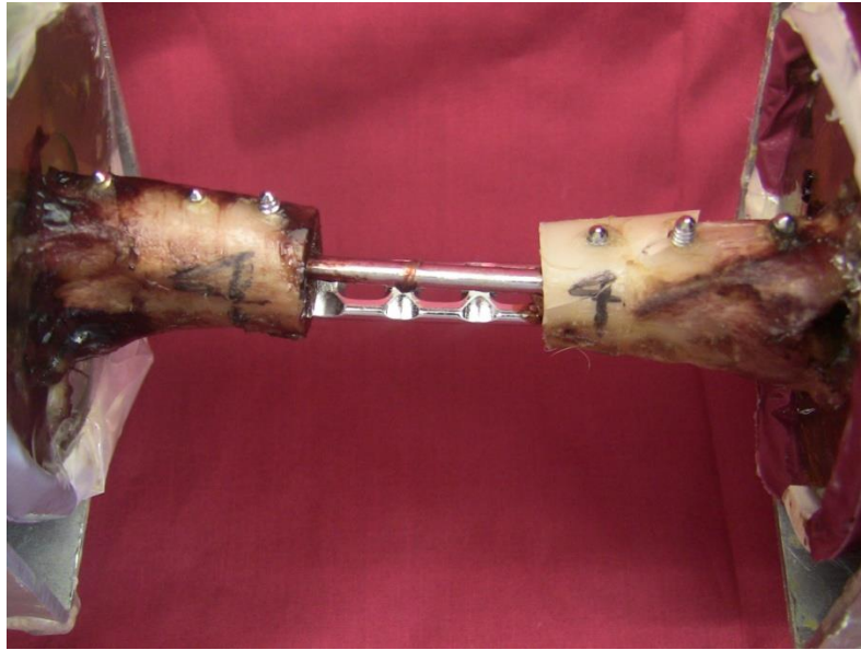
Figure 40. Fracture of LC-DCP #4 where crack initiates at gap and moves to second bone screw hole on transcortex.
