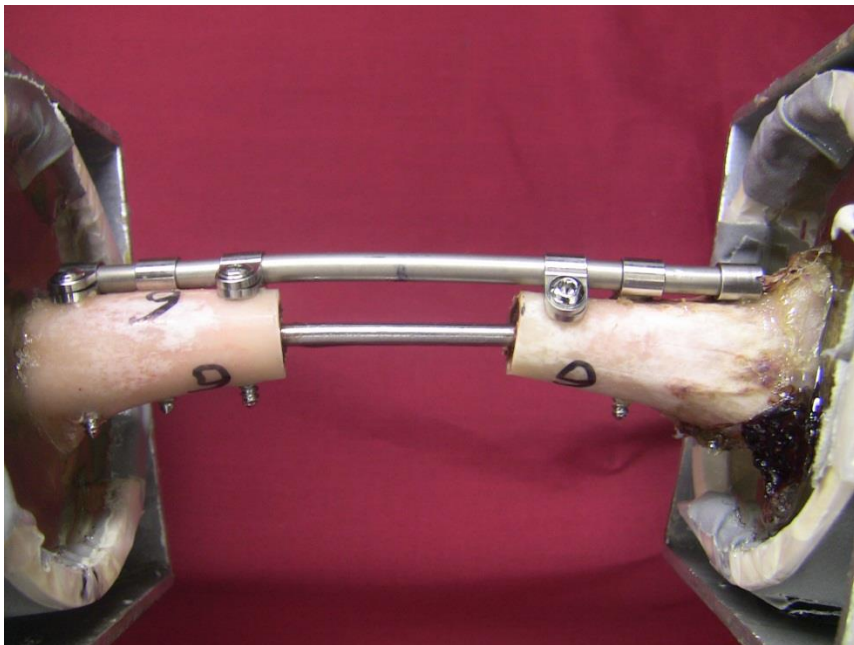
Figure 51. CRIF #6 after four point bending experiment.
