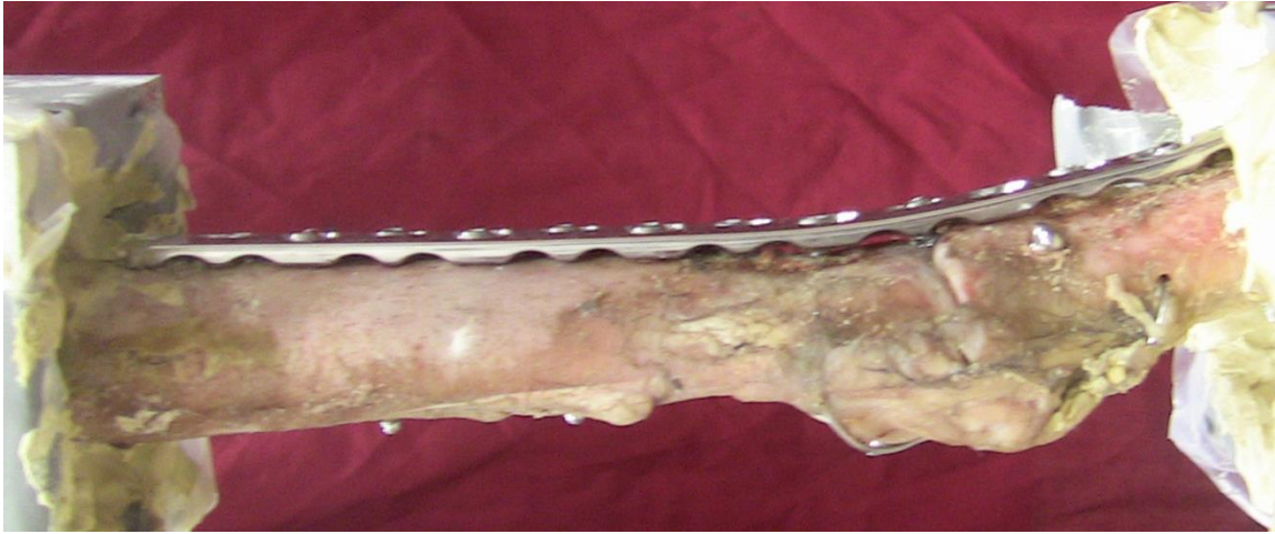
Figure 78. LCP #4 before the single ramp to failure test.
