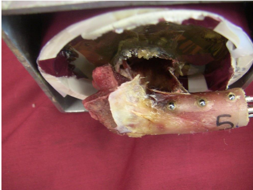
Figure 46. After four point bending test during inspection of LC-DCP #5 the bone separated into two distinct pieces, the portion connected to the plate and the portion attached to the epoxy.
