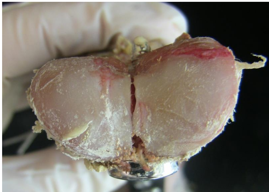
Figure 77. LCP #3 after the single ramp to failure test. This image shows the distal end of the proximal phalanx bone where fracture occurred. The fracture, similar to the other LCP/wire constructs, bisects the bone connecting the locking bone screw holes.
