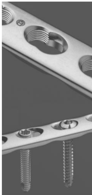
Figure 24. The top half of the image above shows a close up view of the LCP locking and compression screw holes. The smooth surface of the hole represents the cortical bone screw surface, where the threaded portion is used for the locking screws. The bottom half of the image shows a locking screw on the left and a cortical bone screw on the right. (23)
