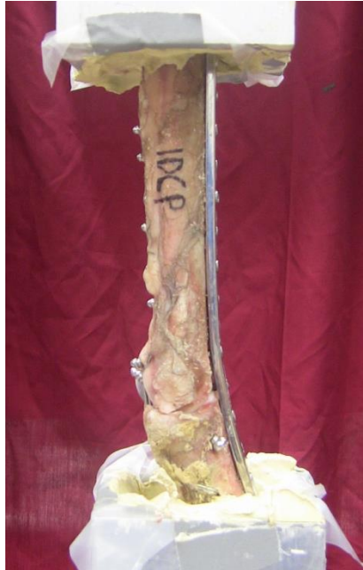
Figure 67. DCP #1 mounted to the MTS 810. Image is used to detail angle in plate before single ramp to failure test.
