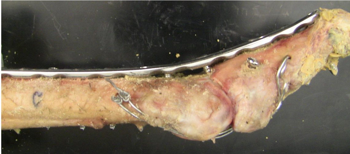
Figure 74. LCP #2 before the single ramp to failure run. This image partnered with Figure 75 helps to show how the LCP constructs suffered from significantly less permanent deformation of the plate by observing the limited change in angle of the plate.
