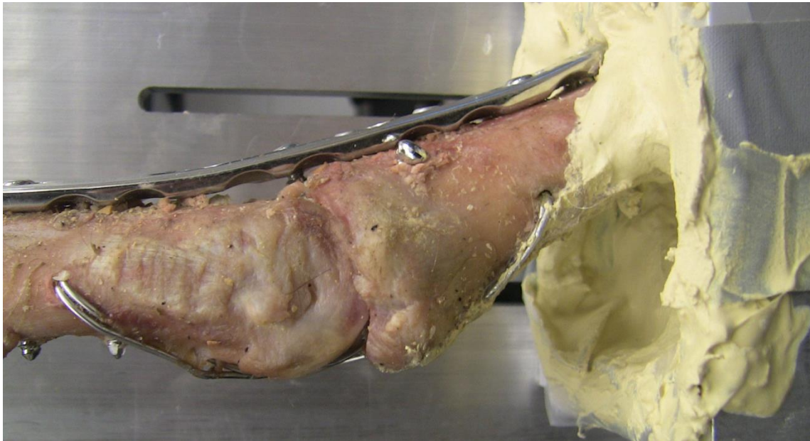
Figure 74. LCP #2 before the single ramp to failure run. This image partnered with Figure 75 helps to show how the LCP constructs suffered from significantly less permanent deformation of the plate by observing the limited change in angle of the plate.
