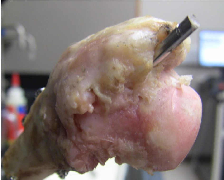
Figure 23. This image shows the IM pin pressing through the femoral neck region after a buckling experiment. This result is one of the main reasons for pursuing a four point bend test.
