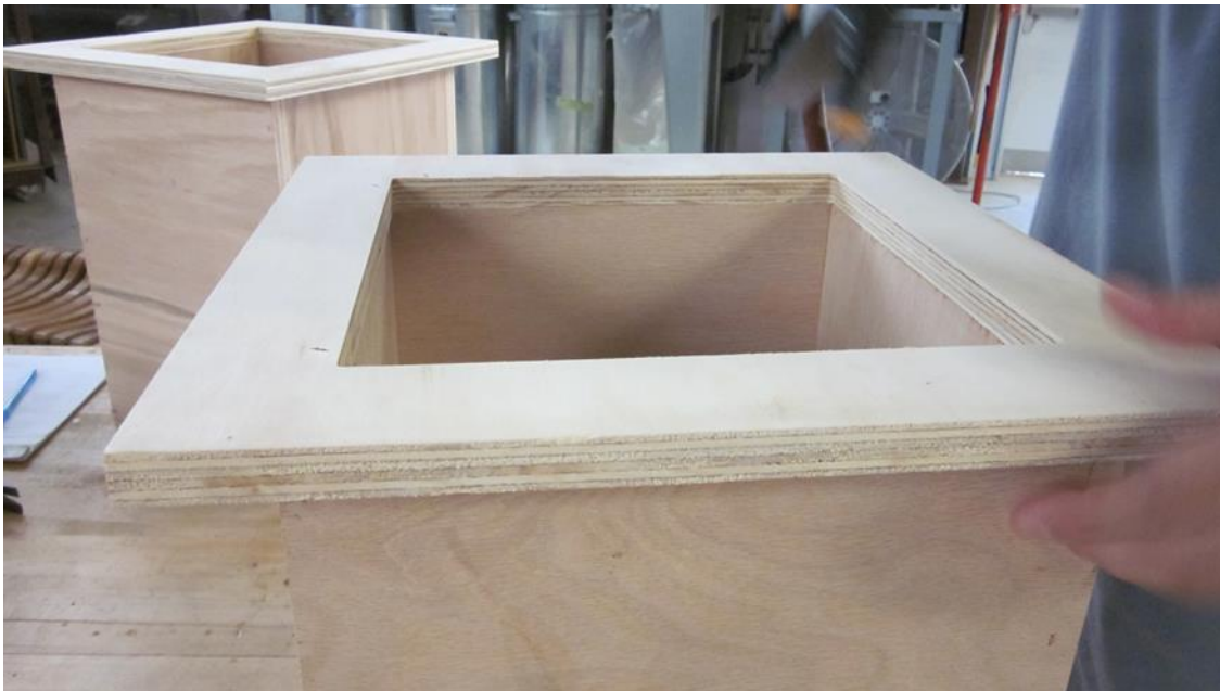
Figure 17 Flange pieces attached to Containments A and B
