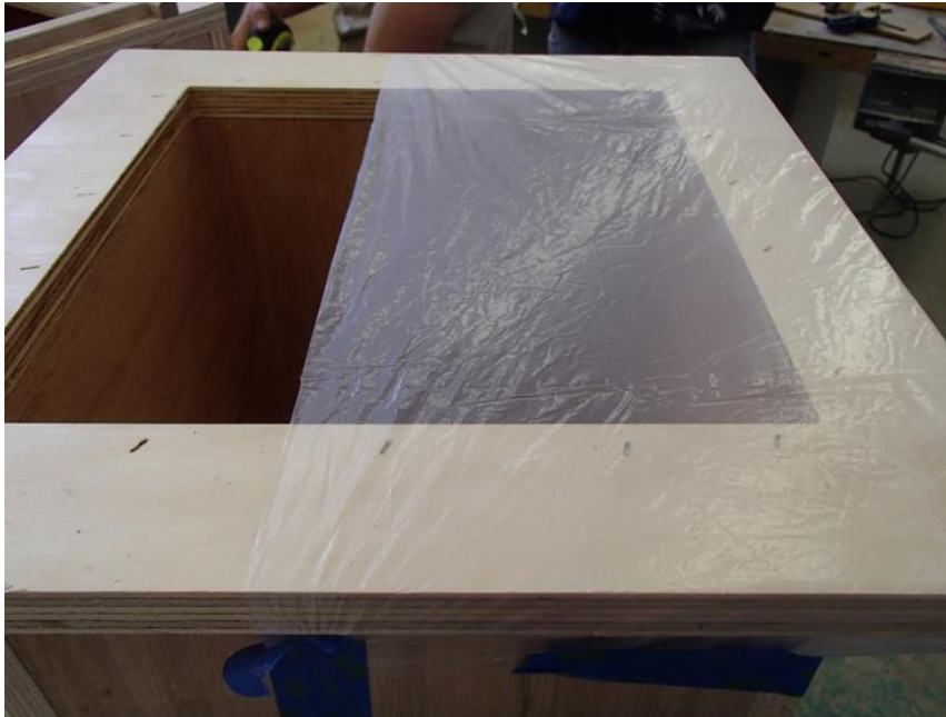
Figure 26 Placement of first plastic sheet
