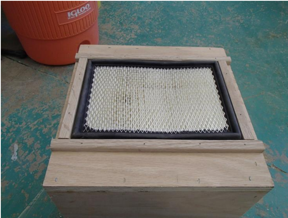
Figure 20 Filter fitted into place in containment vessel
