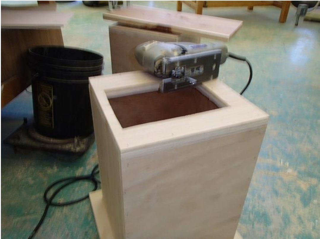
Figure 19 Filter space being cut into the containment vessel
