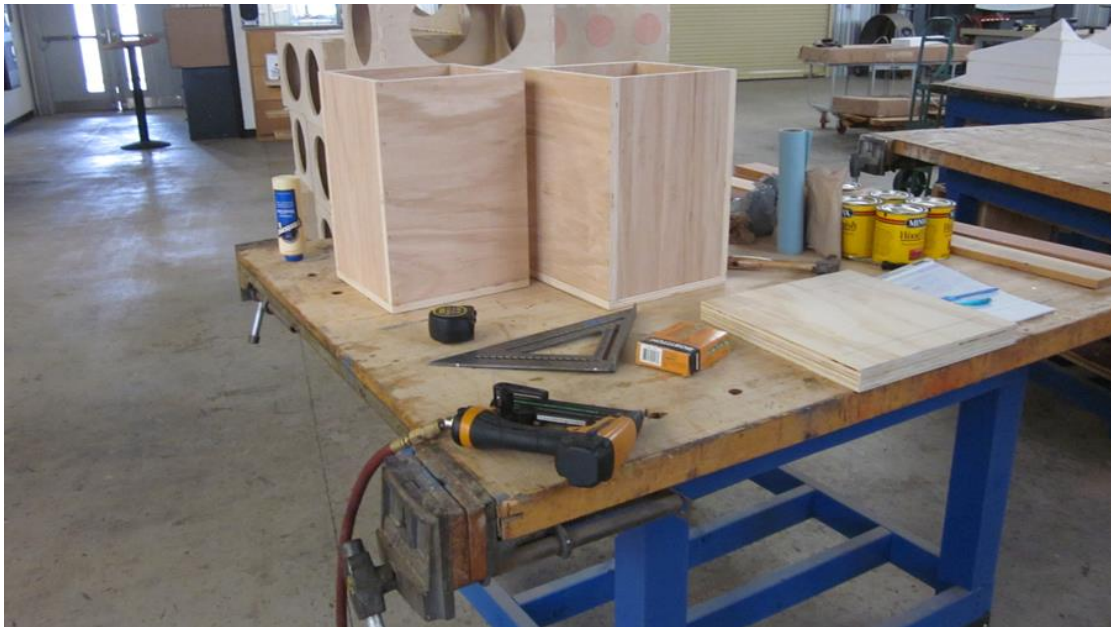
Figure 15 Containment A and Containment B without flange pieces
