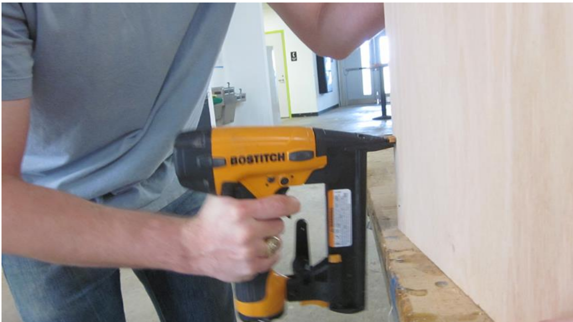
Figure 12 Nail gun used to hold boxes until glue dries
