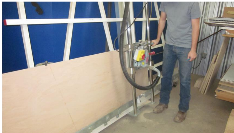
Figure 8 Panel saw cutting plywood
