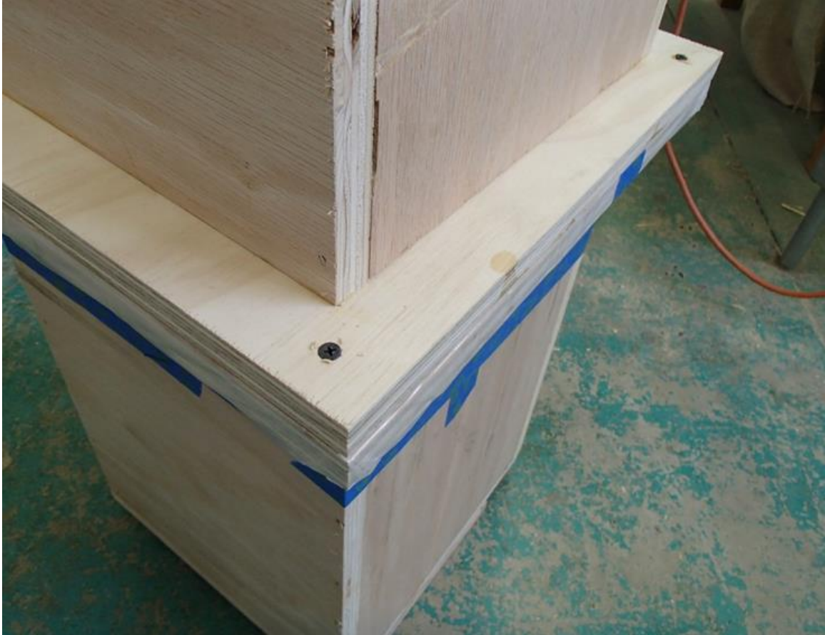
Figure 29 Flanges secured with screws
