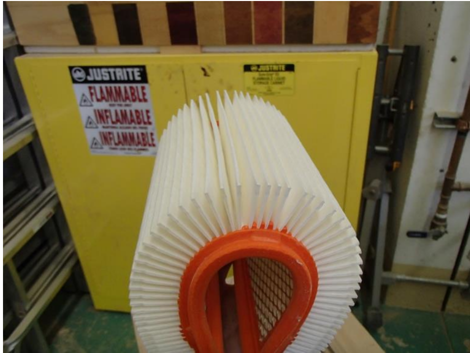
Figure 37 Filter removed after eighteen hours
