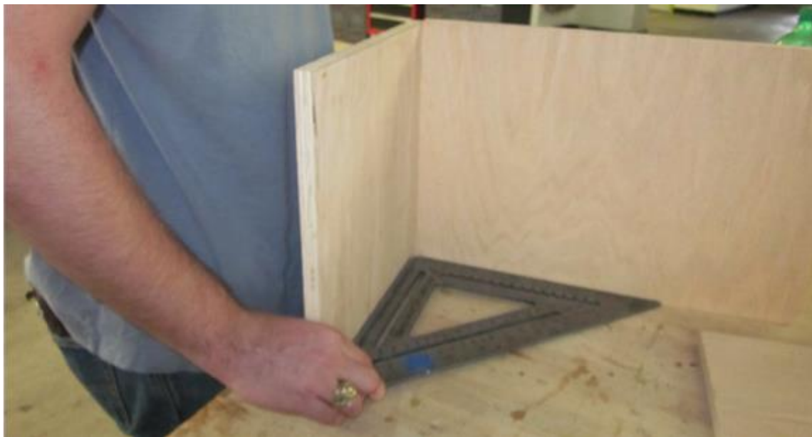
Figure 10 Squaring the plywood box
