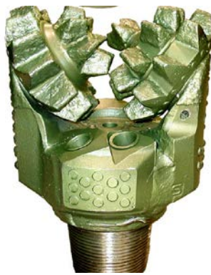
(b) 2-Cone Roller Bit with Large Milled Teeth
