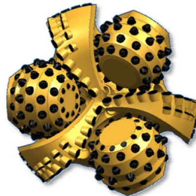
(c) 3-Cone Roller Bit with Small Insert Teeth
