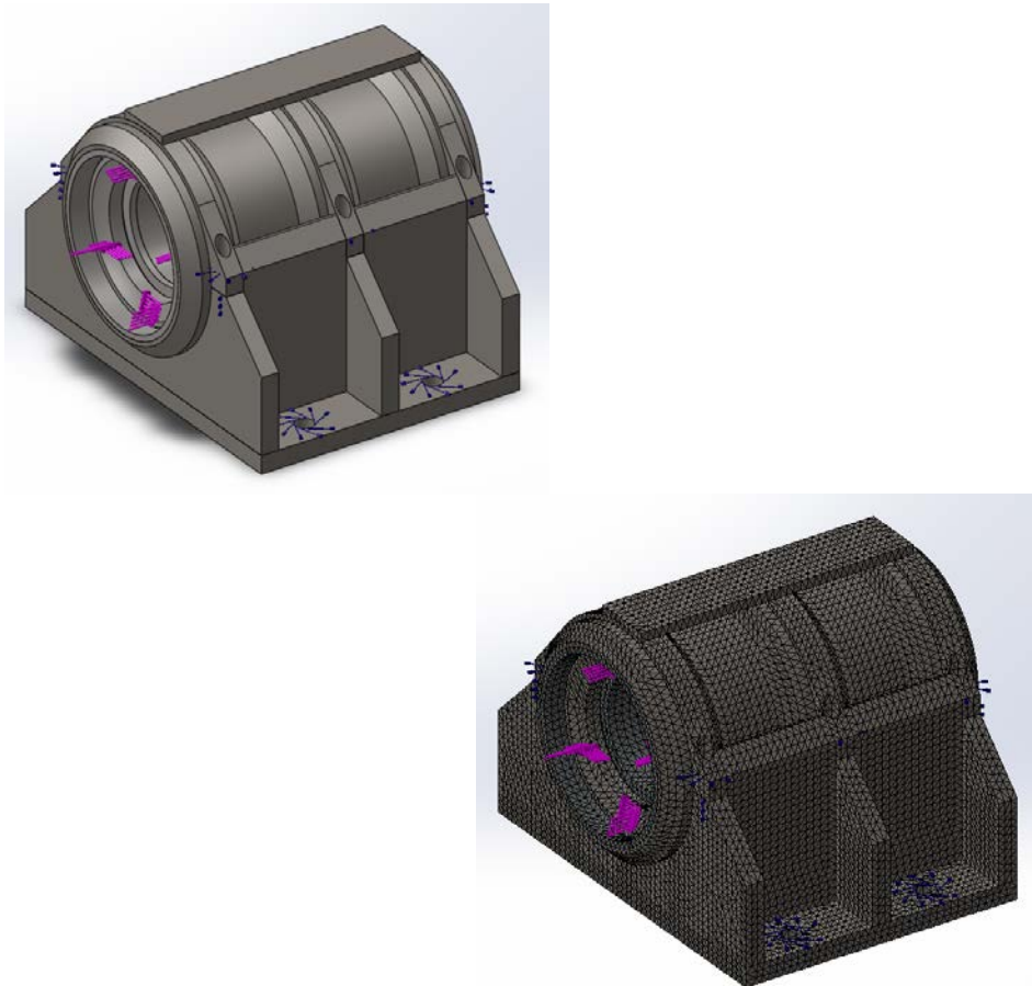
Figure 3.58: CAD Model and Mesh Plot for Shaft Support
