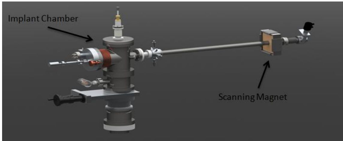
Figure 4.2: Close up 3D model of the implant chamber and the scanning magnets.
