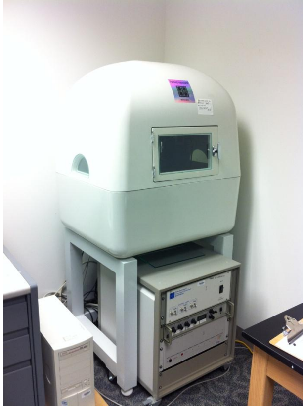
Figure 4.3: Photograph of the nanoindenter used for this experiment at Texas A&M University.
