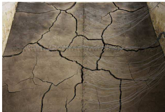
Figure 1.2. An image of the slope of the scaled embankment after a drying cycle
