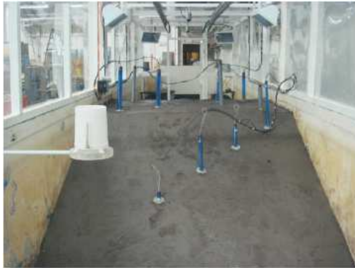
Figure 4.4. Picture of the scaled embankment inside the environment chamber
