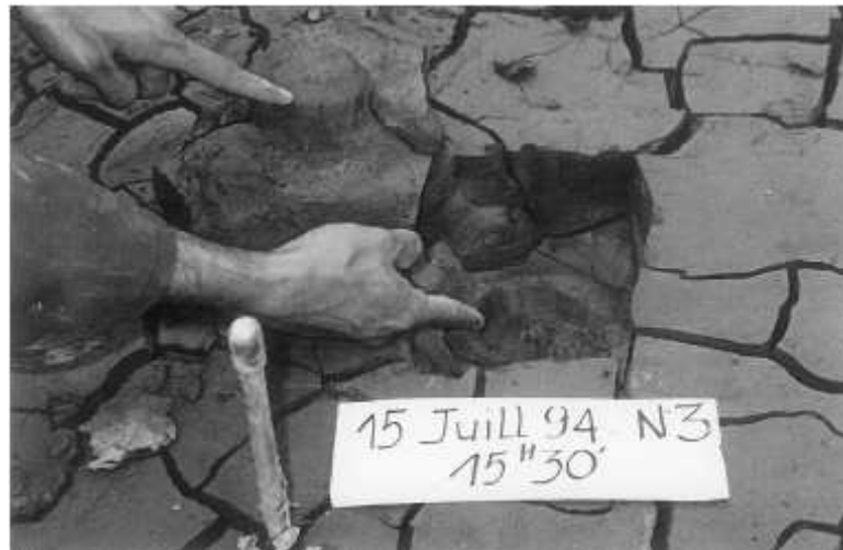
Figure 2.5. Picture depicting polygonal cracking with protuberance (after Konrad and Ayad, 1997)
