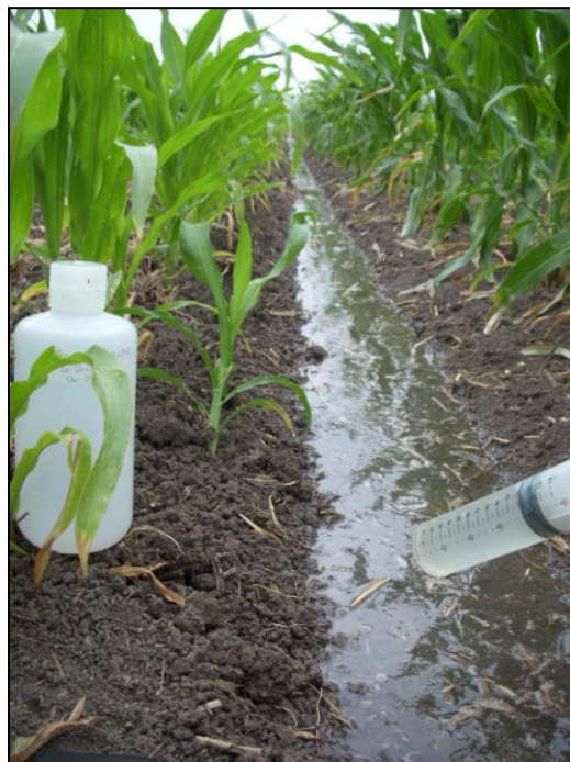
Figure 15. Collecting a water sample from initial runoff with a syringe at the end of the furrow.
