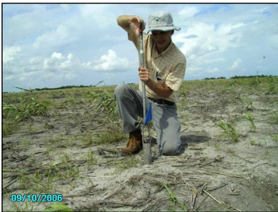
Figure 18. Left: Installing a piezometer to obtain groundwater samples. Right: Probe to measure the depth of the water table.
