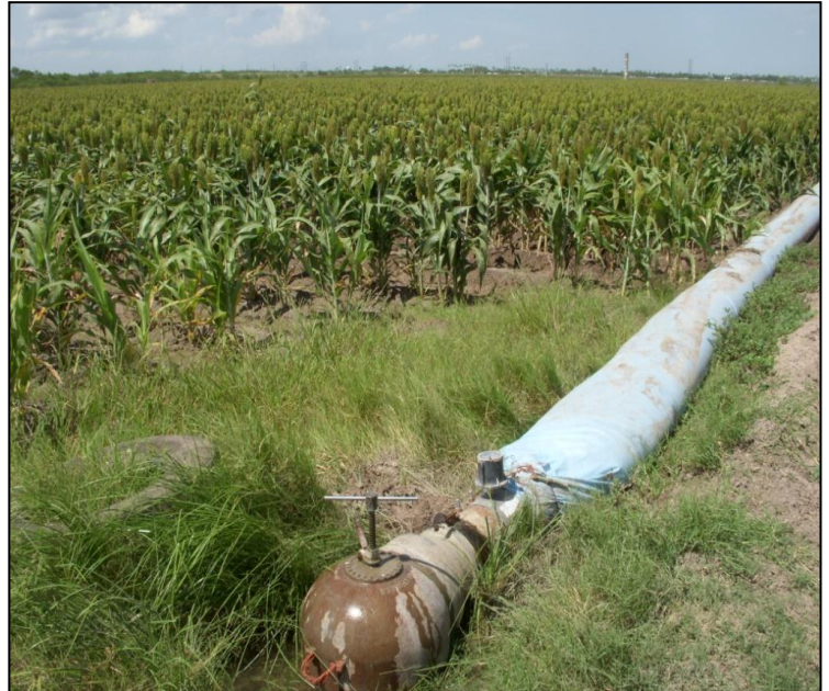
Figure 10. Propeller flow meters used to measure irrigation depth.
