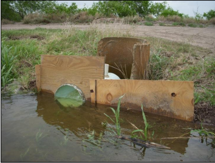
Figure 14. Left: Circular flume measuring runoff with a data logger. Right: Hydrograph obtained during the irrigation event.
