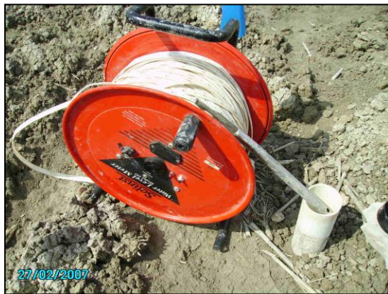
Figure 18. Left: Installing a piezometer to obtain groundwater samples. Right: Probe to measure the depth of the water table.
