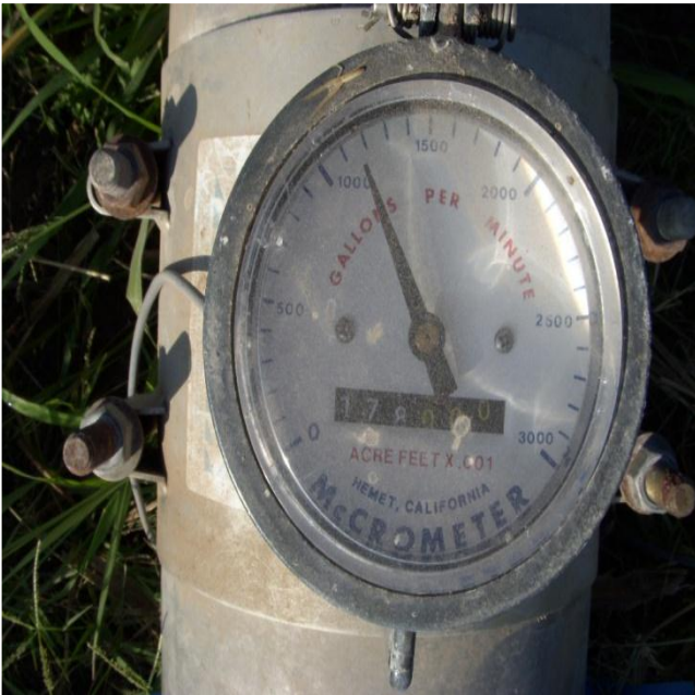
Figure 10. Propeller flow meters used to measure irrigation depth.
