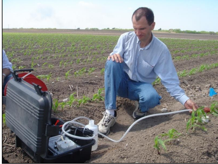
Figure 19. Collecting a groundwater sample with a variable flow pump from a 2-inch well.
