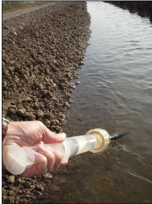
Figure 16. Collecting a water sample to determine peak runoff.
