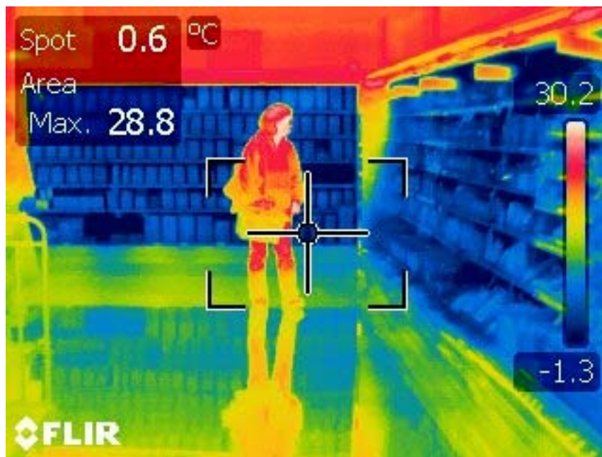
Fig. 8. An infrared image showing cold aisle conditions for customers
