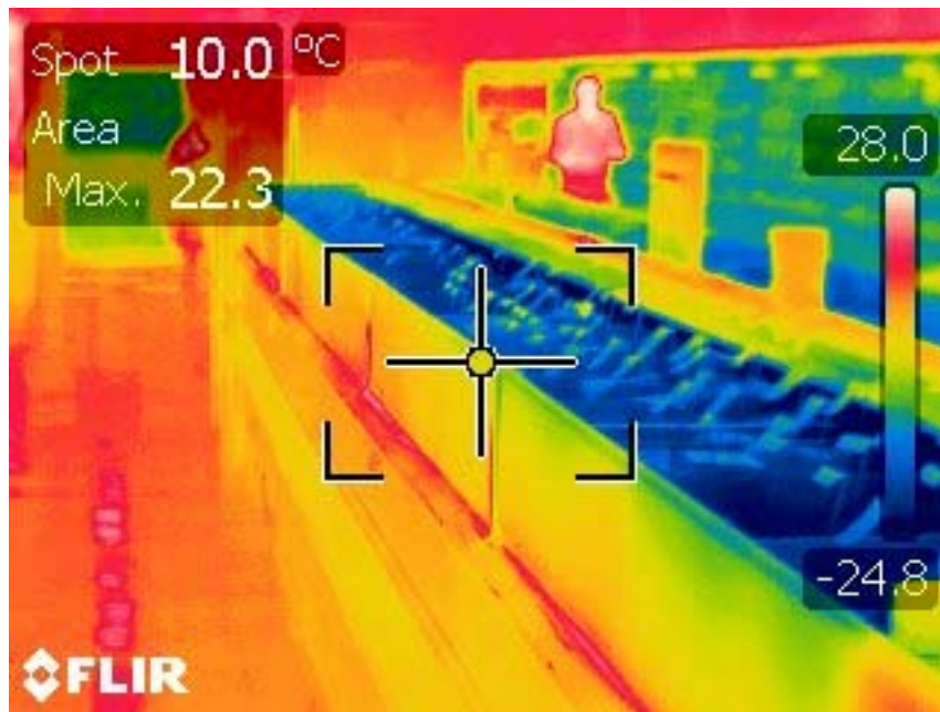
Fig. 11. The aisle is noticeably warmer next to tough freezer because less cold air escapes
