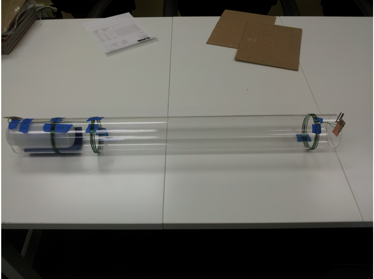
Fig. III.7. Former with both gradiometer and single loop coils. The water bottle phantom used for test imaging is inside the gradiometer coil.
