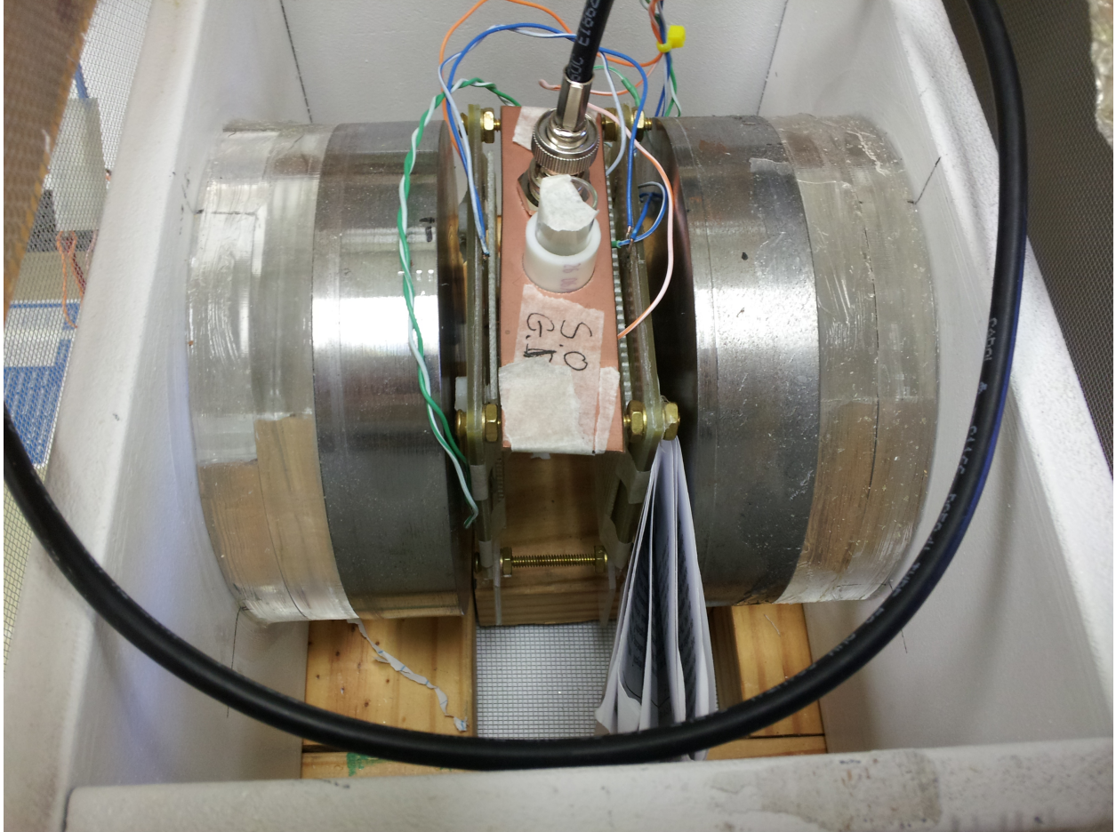
Fig. II.2. Magnet, gradients, and RF coil of desktop imaging system
