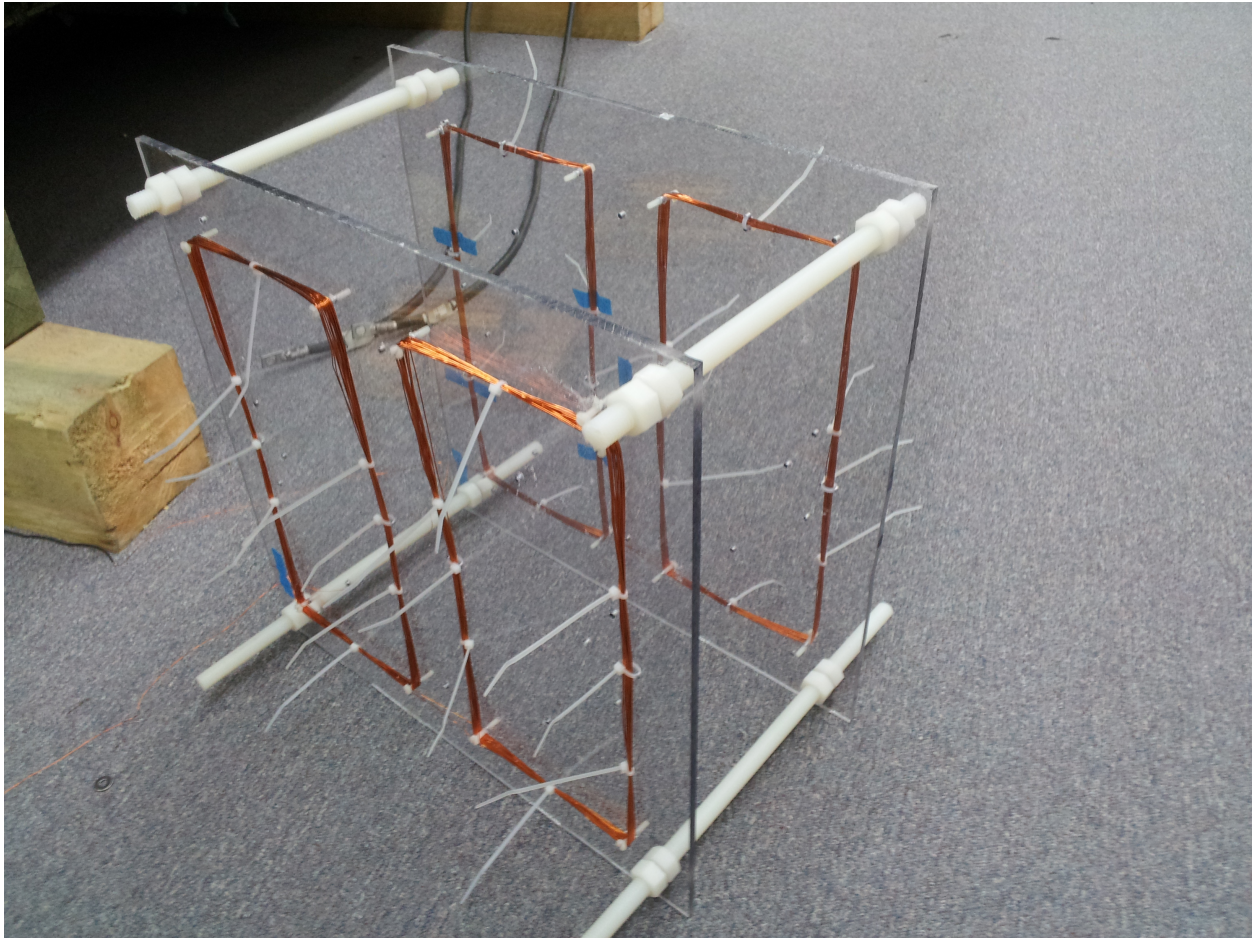
Fig. III.6. Single-axis gradient set as constructed
