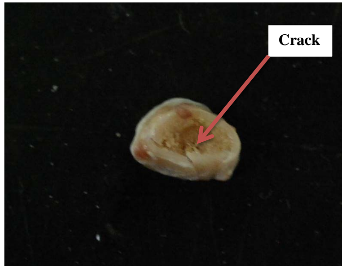
FIG. 9. A representative axially-loaded bone specimen after failure.
