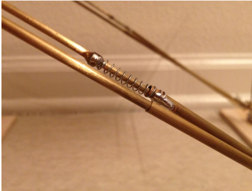
Fig. 28. In-plane bracing with spring element and friction damper
