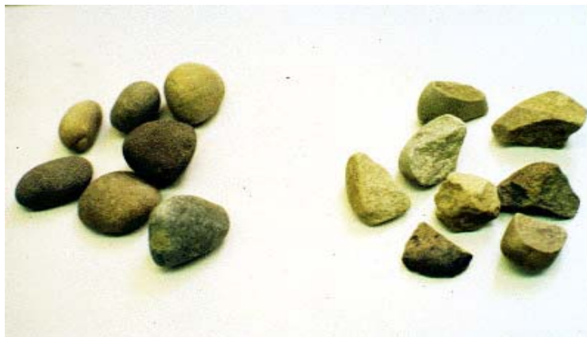
Fig. 2.12. Illustration of Counting Percent of Fractured Faces
