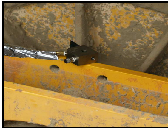
Fig. 3-2. Accelerometer mounted on roller.
