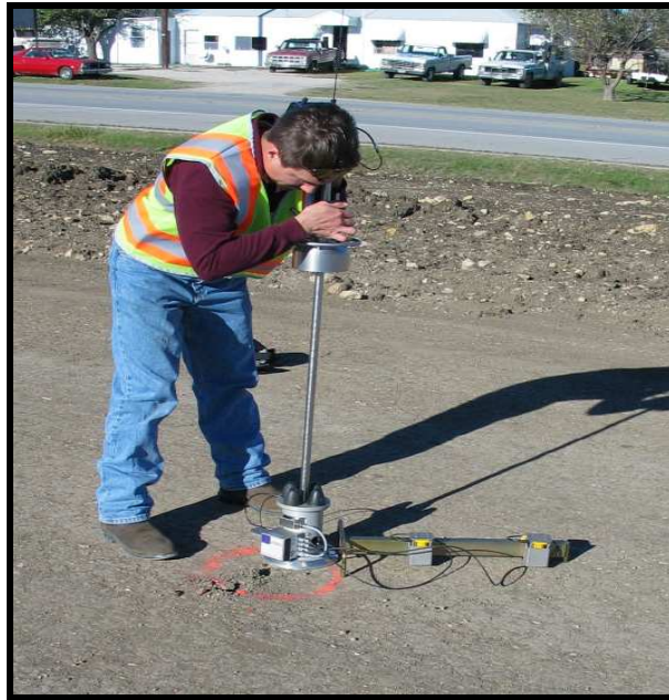
Fig. 4-3. Portable falling weight deflectometer. Photograph courtesy of Dr. Wenting Liu.
