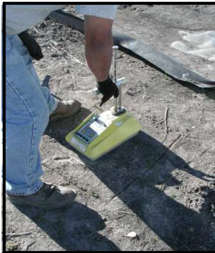
Fig. 4-1. Nuclear gauge. Photograph courtesy of Dr. Wenting Liu.
