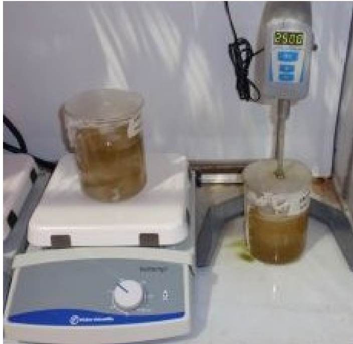
Figure 2. Test setup for initial shear testing of diatoms.
