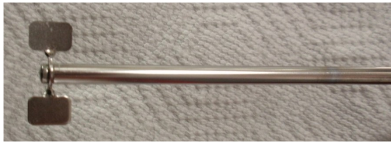
Figure 1: Cole Parmer 30mm diameter straight impeller used in the laboratory mixer for initial shear testing
