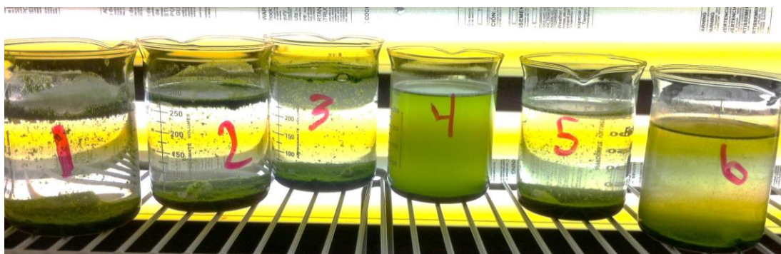
Figure 10: Photo of results from polymer tests (flasks 1-3: no polymer addition, flasks 4-6: treated with polymer flocculant)
