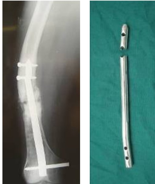
Figure 53. The x-ray and regular image show the bend in the short femoral intramedullary nail.
