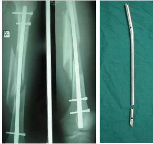
Figure 55. The x-ray and regular image show the bend in the tibial intramedullary nail.
