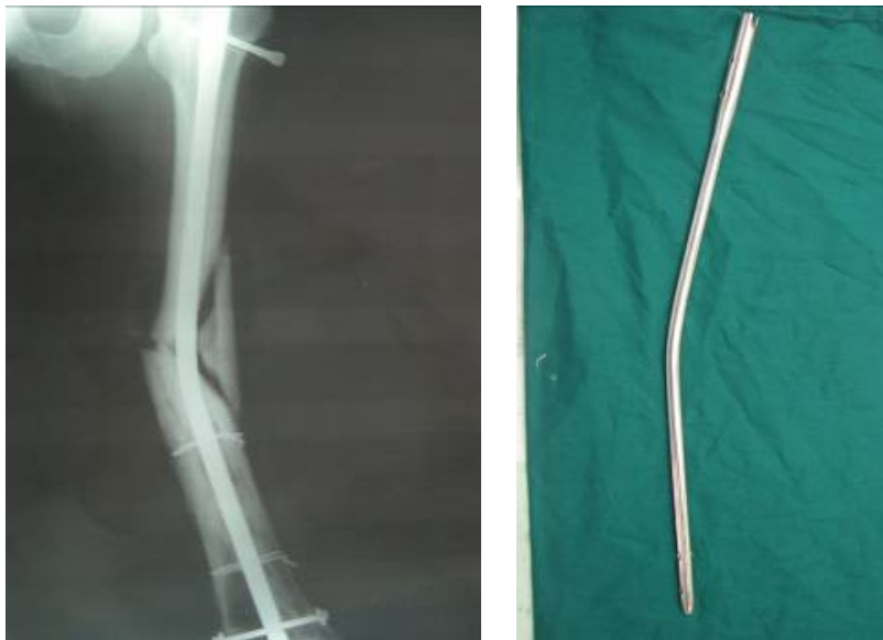
Figure 52. The x-ray and regular image show the bend in the long femoral intramedullary nail.
