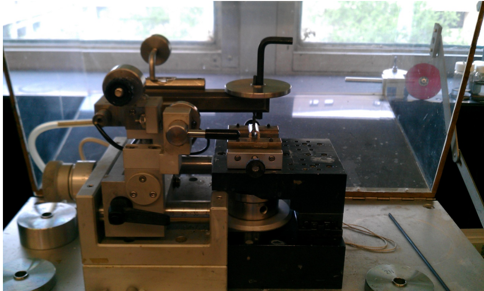
Figure 24. The tribometer doubled as a scratch tester when a drill bit was used in place of a ball bearing.
