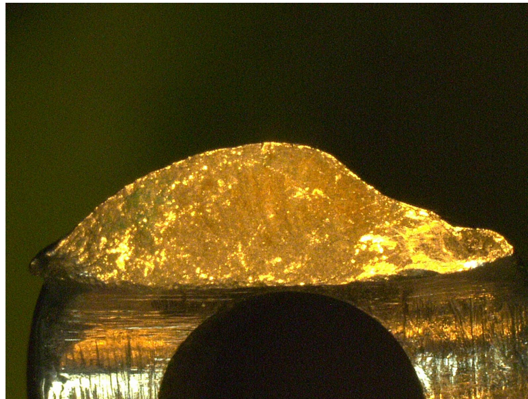
Figure 54. The fractography shows a brittle fracture.
