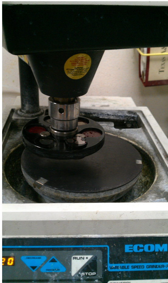
Figure 29. The samples were placed in a fixture, which attached to the rotating polishing head.
