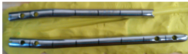
Figure 44. The roughness average data for the short femoral nails shows no conclusive evidence for a difference, but it appears that the implanted sample is rougher on average.
