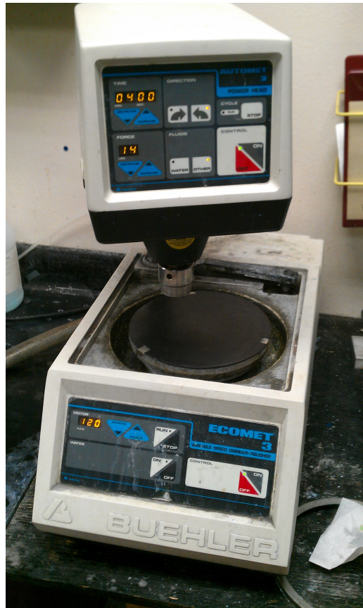
Figure 28. The Automet 2 polishing head mounts on the Ecomet 3 polishing table. Each machine is equipped with controls that are integrated with the other.
