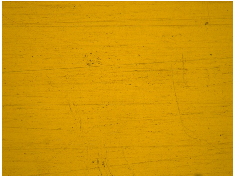
Figure 49. The non-implanted stainless steel appears to be polished although having several scratches.
