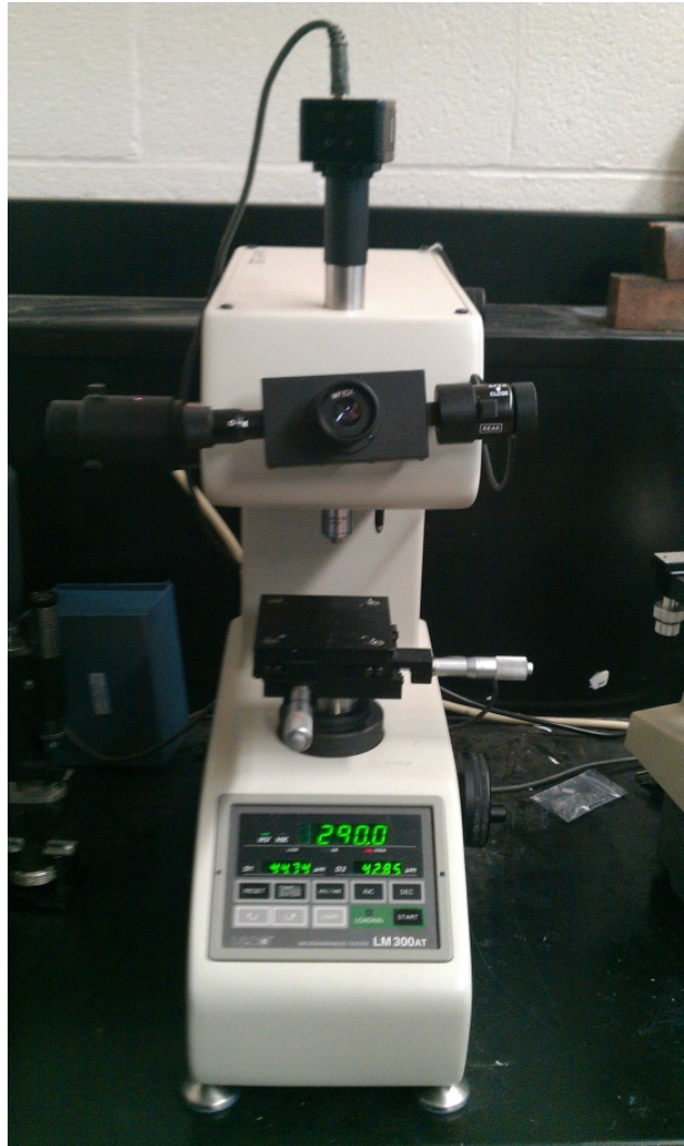
Figure 16. The LM 300 series Vicker's microhardness indenter was used to test the materials' hardness.
