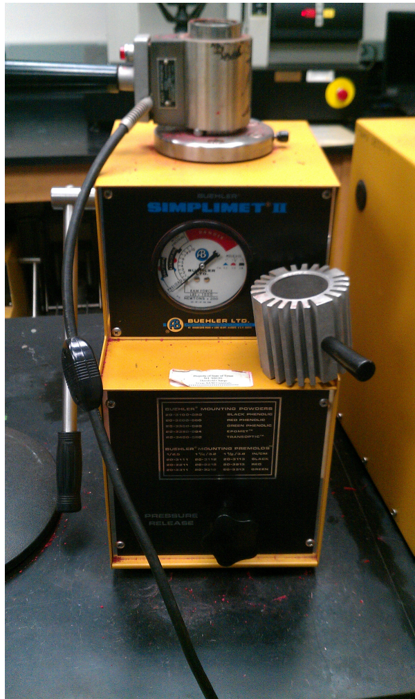
Figure 27. The Simplimet mounting press machine comes equipped with a pressure gauge, a heating cylinder, and cooling fins.
