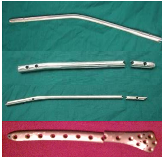
Figure 13. The tested samples supplied by the Shandon Hospital in order from top to bottom: long femoral nail, short femoral nail, tibial nail, femoral plate.
