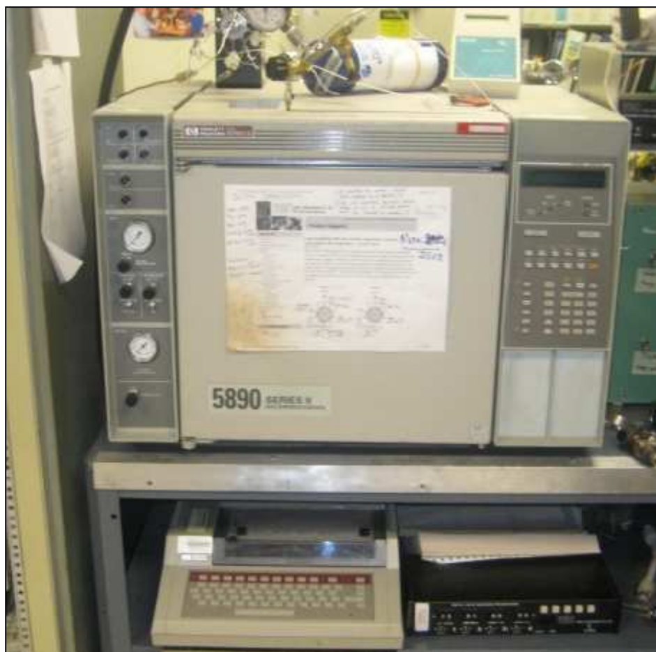
Fig. 11- Laboratory gas chromatograph. Produced gas was analyzed for carbon dioxide, oxygen, nitrogen, and carbon monoxide.
