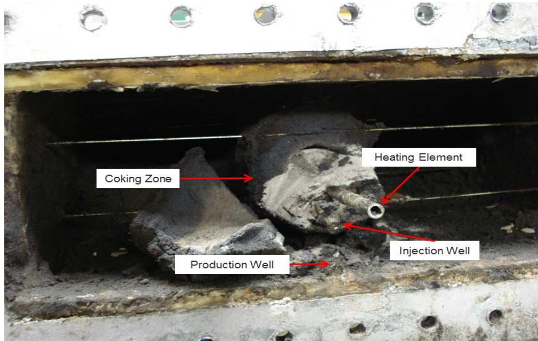
Fig. 19- Post-experiment sand-pack analysis. A cylindrical shape coke zone with thickness of about 3 cm formed around injector and the electrical heart. (Run 1)
