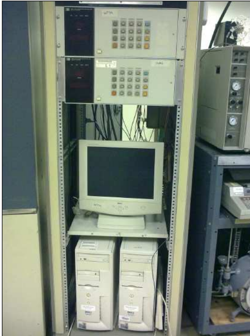
Fig. 16- Production data logger. Cumulative gas production was recorded by using this data logger
