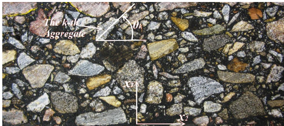
Figure 3-1 Vertical section of an asphalt mixture field core showing aggregate orientation
