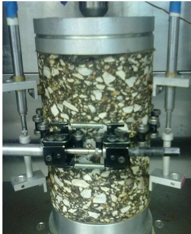
Figure 7-4 Testing configurations of the UCC, NDM, DDM tests including axial and radial LVDTs.
