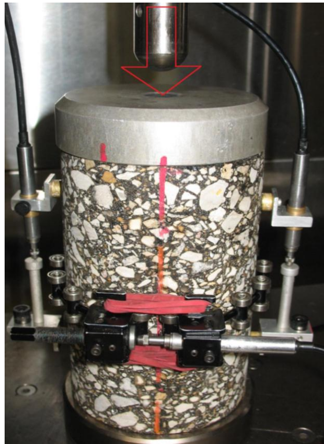
Figure 2-3 Configuration of the compressive creep test
