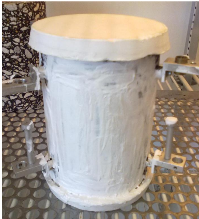
Figure 7-1 An asphalt mixture specimen painted by white plaster on surfaces before destructive test
