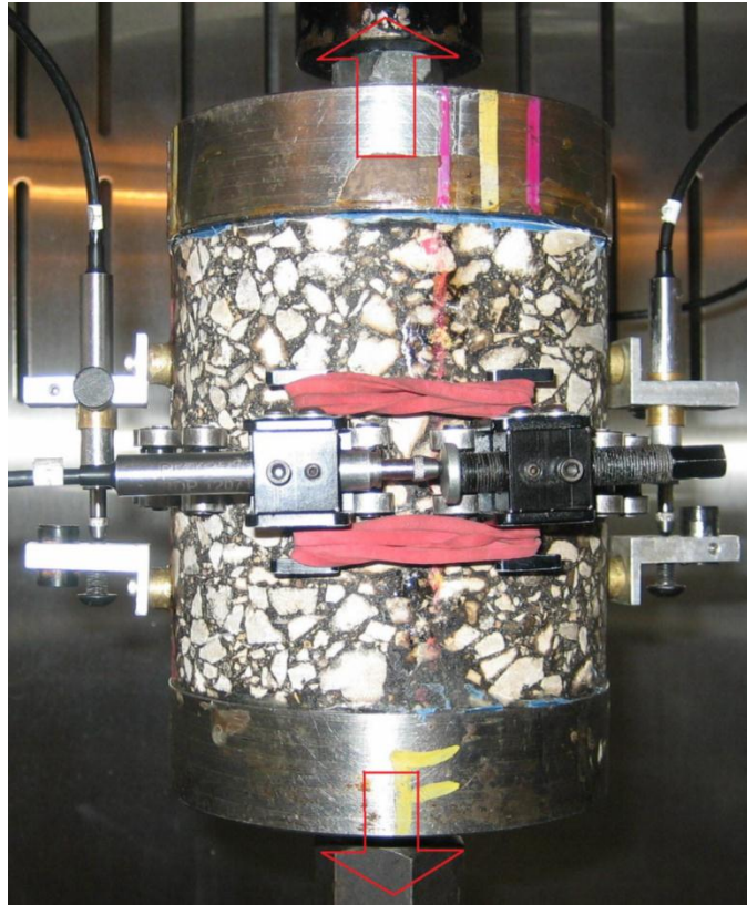
Figure 2-11 Configuration of the uniaxial tensile creep test
