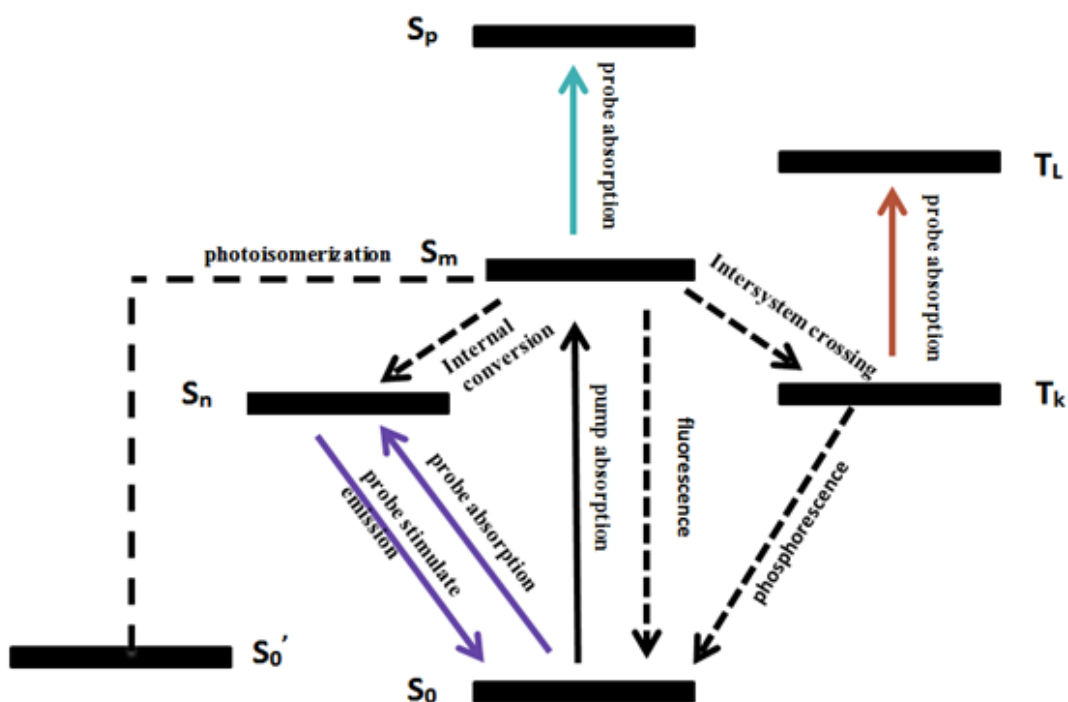
Figure 2. Multilevel energy level diagram showing various possible transitions accessible through pump-probe techniques.
