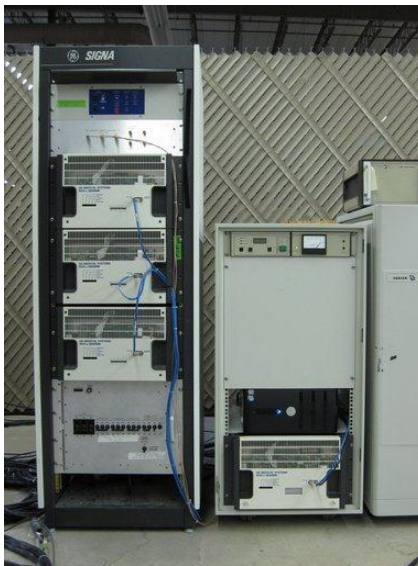
Fig. 41. Fourth gradient controller PC and amplifier. Shown to the right of the standard three-axis gradient amplifier system (since upgraded).
