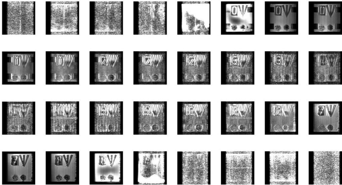
Fig. 63. Resolution enhanced 3D reconstruction using two k -lines. The k -lines are separated by the same distance yielding minimal artifact power in the dual slice experiment above (lines 118 and 138) with the fourth gradient producing a variation of \pm 12 rad/cm over a 1 cm slab. While these lines yield resolution enhanced images from the outer slices, the middle slices yield little signal, as they require lower phase compensation values.
