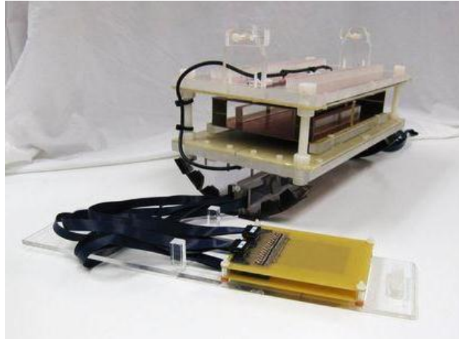
Fig. 36. Photograph of wide field of view imaging probe. The probe consists of the biplanar gradient coil and acrylic former with integrated volume RF excitation coil, shown with the dual sided receive array and loading platform removed [79].
