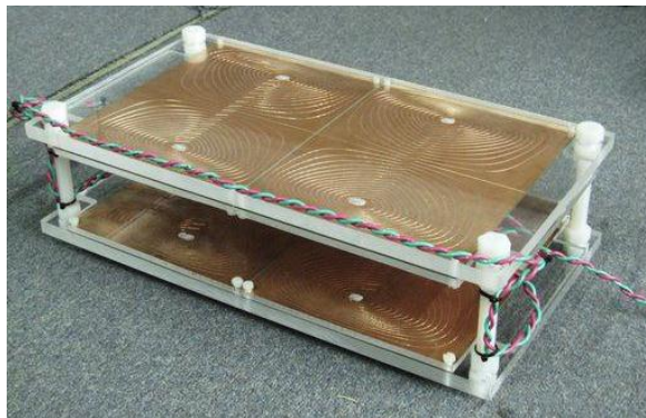
Fig. 21. Prototype biplanar target field gradient coil before integration into an imaging probe.
