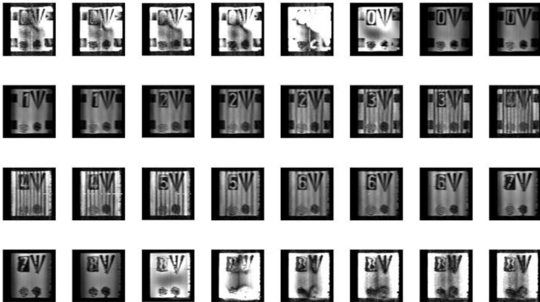
Fig. 65. Artifacts in 3D imaging with the fourth gradient due insufficient coverage of y k -space. Resolution enhanced reconstruction using the same fourth x k -lines above, with the fourth gradient producing a variation of \pm 12 rad/cm over a 1 cm slab but retaining only 32 of the 64 k -line collected. Loss of field of view along x is apparent.
