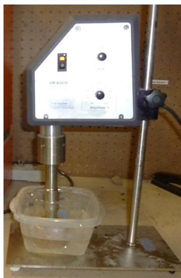
Fig. 2.2. Ultrasonication equipment used for pretreatment.
