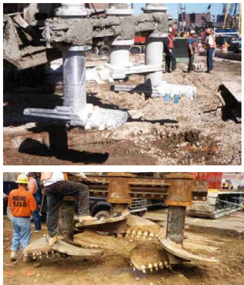
(b) M250 Auger Configurations [Photos after Jakiel (2000)]
