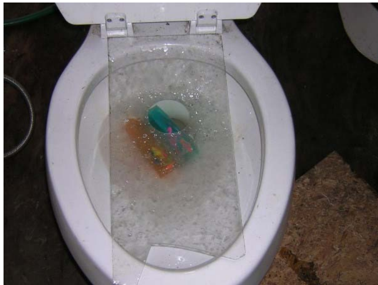
Figure 7: Water Closet Bowl with Plastic Plate and Media
