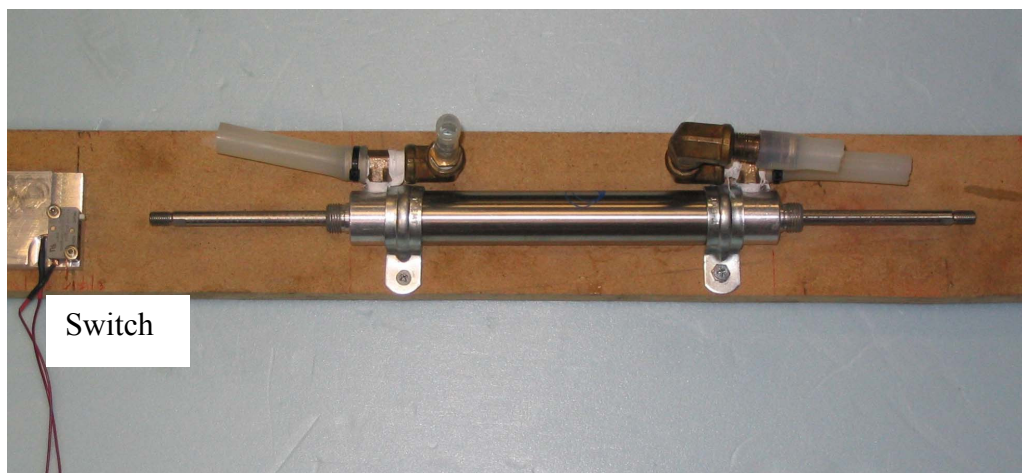
Figure 21. Double-rod double-acting cylinder and switch.
