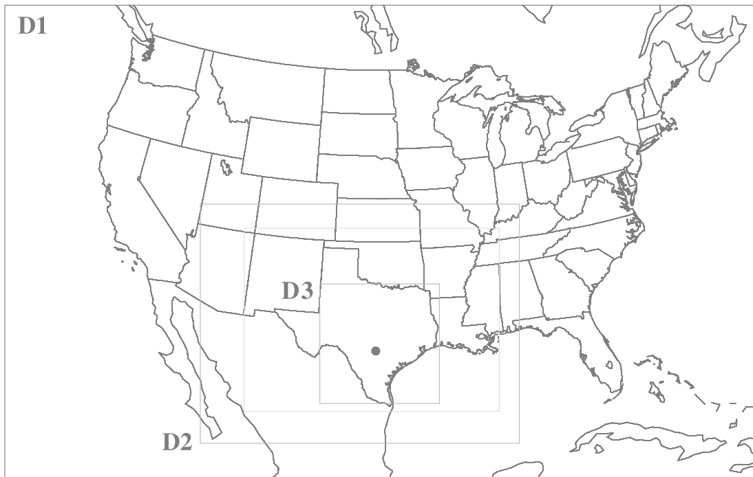
Fig. 3.1 The relative locations of MM5 model domains. The grid resolutions of D1, D2, and D3 are 30, 10, and 3.3 km, respectively.
