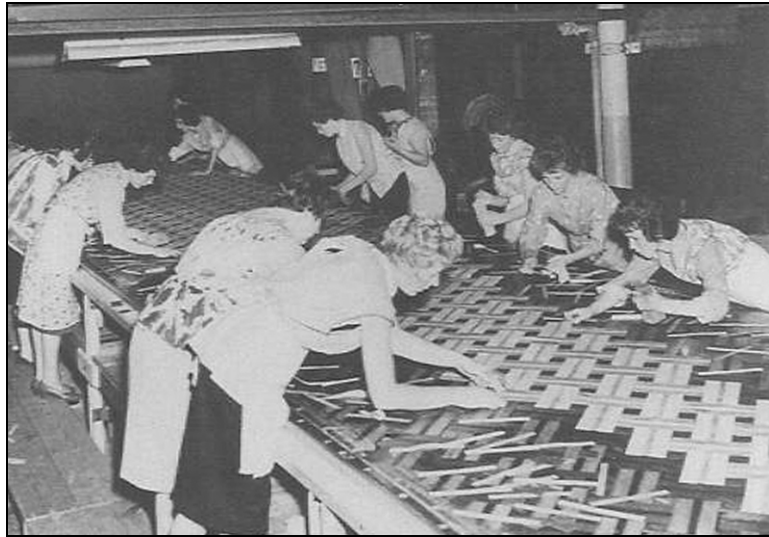
Figure 17. Workers Hand Piecing Inlaid Linoleum Design (after Simpson 1999a:86)
