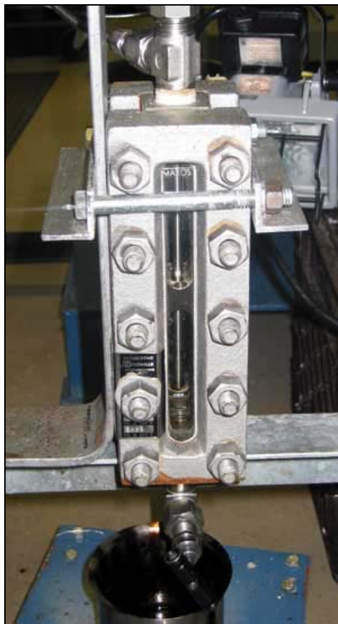
Fig. 3.7— The glass makes it easy to monitor the liquid level in the separator.
