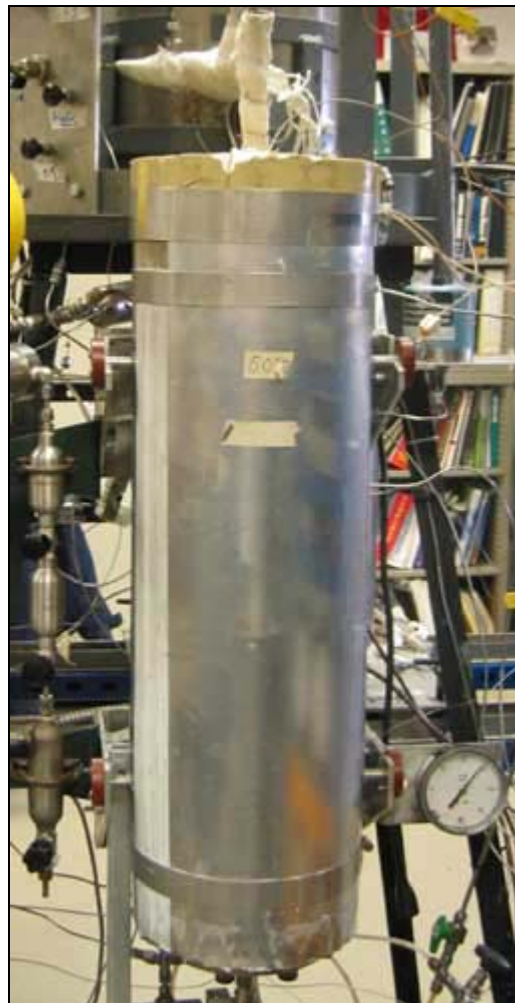
Fig. 3.6— The cell is placed inside a heating jacket.
