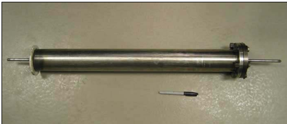
Fig. 3.4— The sand mix is contained within this cylindrical cell.
