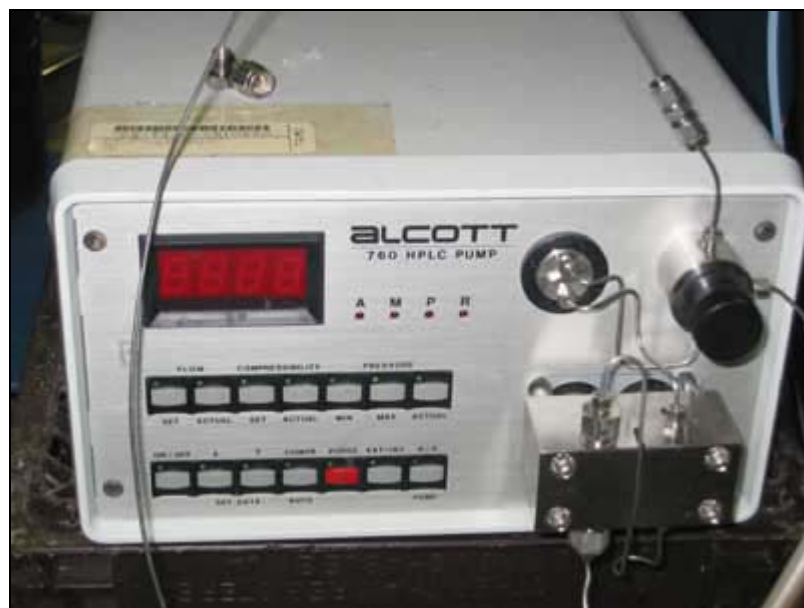
Fig. 3.2— HPLC pump used for water injection.
