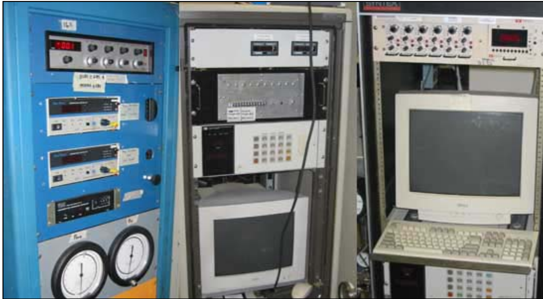
Fig. 3.10— Overview of temperature controllers, data loggers, computers and other electronic equipment used to monitor the experiments.
