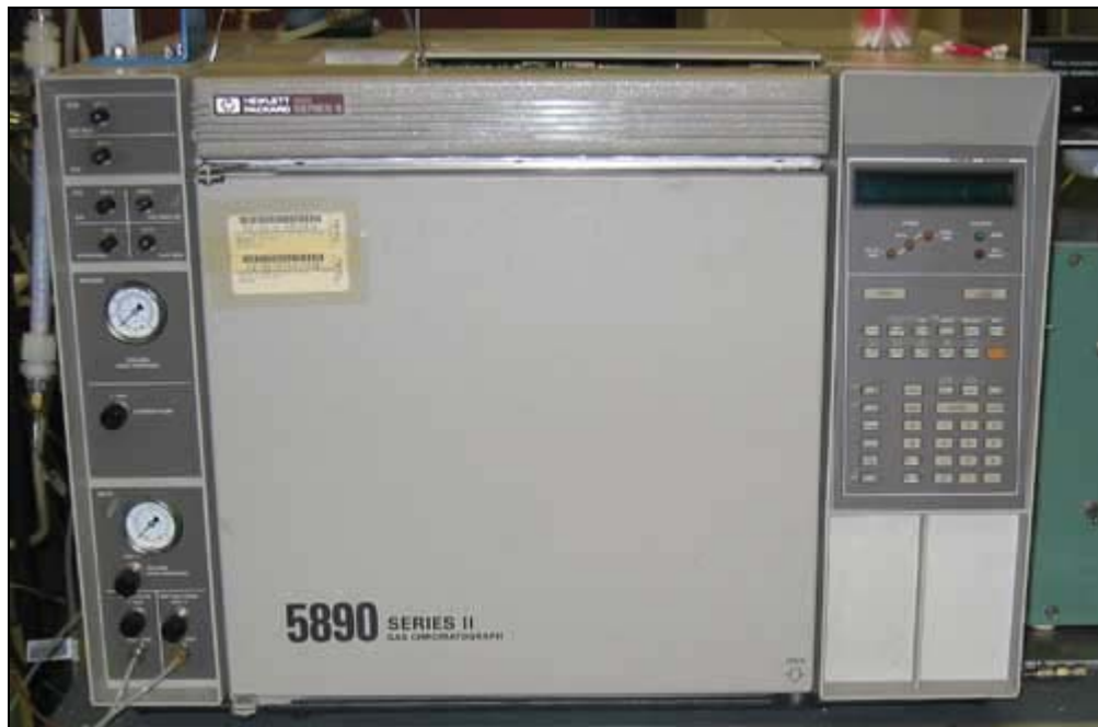
Fig. 3.9— A GC allows the produced gas composition to be measured.
