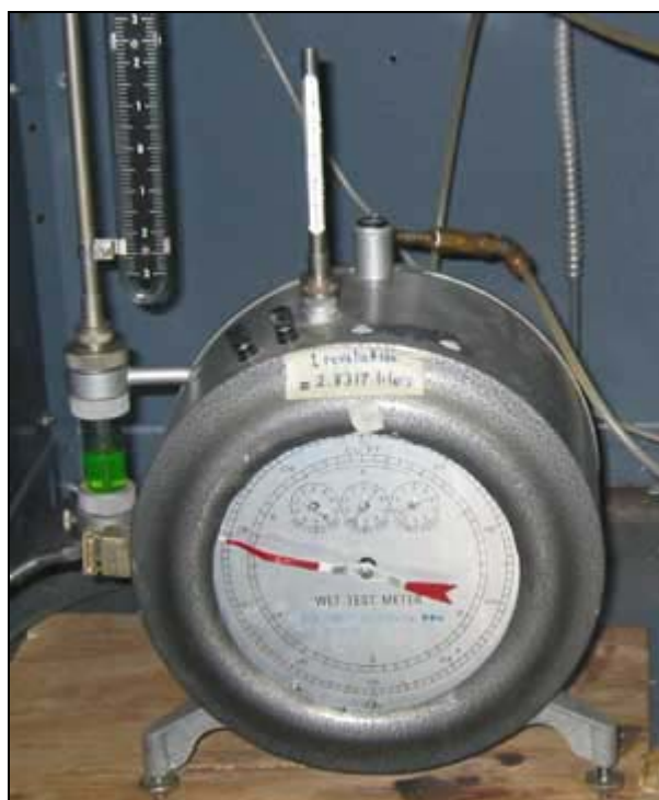
Fig. 3.8— Wet test meter for measuring gas volume.
