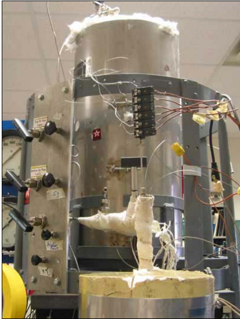
Fig. 3.3— Steam generator, insulated pipes and the thermocouples.
