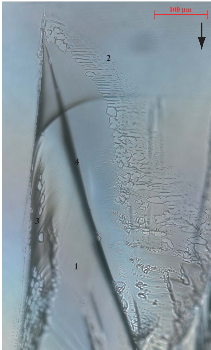
FIGURE 31. Healing of branched cracks in quartz prism 3F#1, annealed at 400°C for 24 hours with distilled water as a pore fluid. The black arrow shows healing direction from the crack tip to the crack initiation point. (1) Large partially healed microcrack out of plane of the main r-crack. The main r-crack is parallel to the photograph, and shows little to no healing. (2) Fluid-filled tubes and fluid inclusion trails formed at the microcrack tip. (3) Healed patches in the transition from healed quartz with fluid inclusions to open crack. (4) High angle microcrack intersecting both the main crack and the partially healed microcrack.
