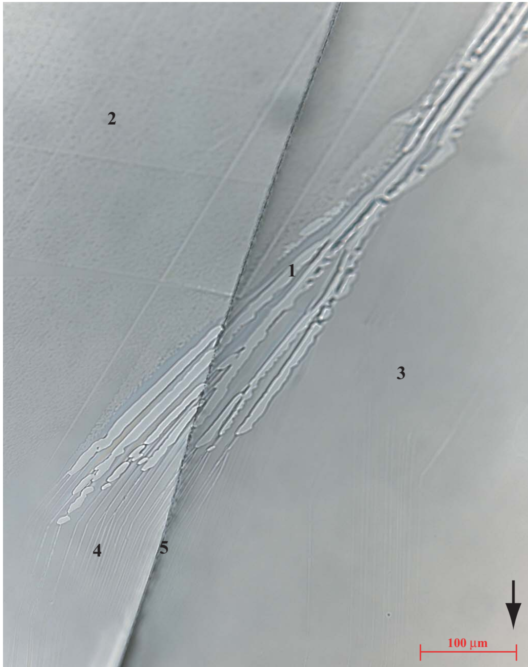
FIGURE 26. Branched quartz bridges formed by enhanced healing of quartz at hackle marks forming a river pattern in quartz prism 2F#2 (annealed at 400°C, 24 hours, with distilled water). The healing direction, from the crack tip to the crack initiation point is shown by the black arrow. (1) A healed hackle mark. (2) Open crack with altered surface. (3) Open crack with less altered surface. (4) Fine scale river pattern that has not healed in the experimental time. (5) Microcrack that formed at a high angle to the r-plane after the start of the experiment.
