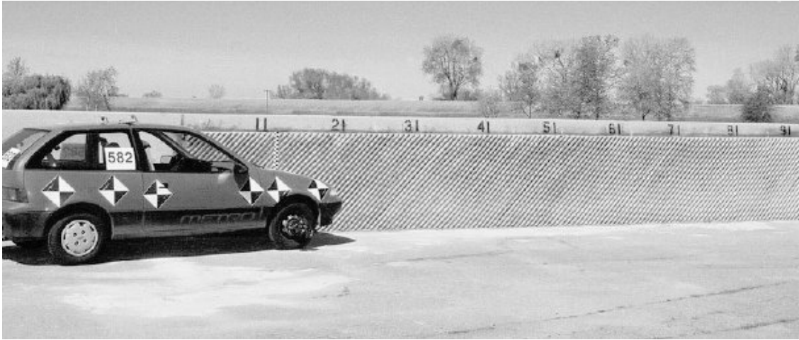
FIG. 9. CalTrans Single Slope Barrier with Fluted Surface Texture (White et al. 2002)
