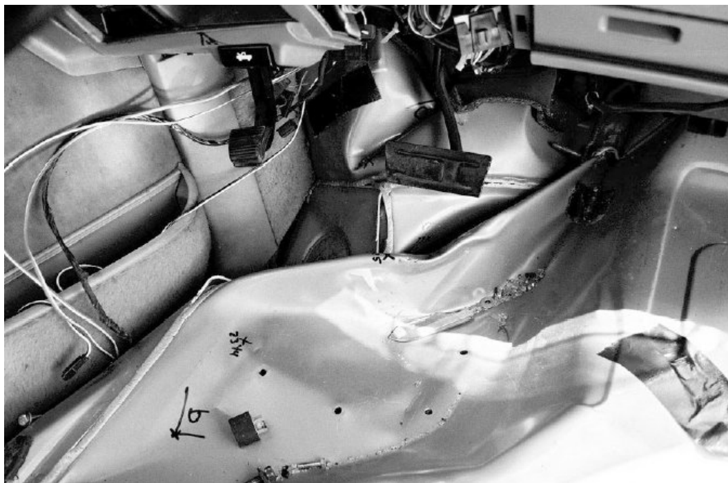
FIG. 18. Occupant Compartment Deformation (White et al. 2002)
