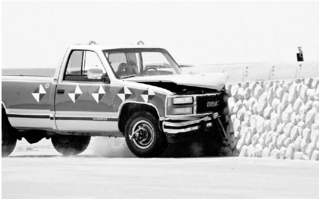
FIG. 3. Single Slope Barrier with Unacceptable Surface Geometry (White et al. 2002)
