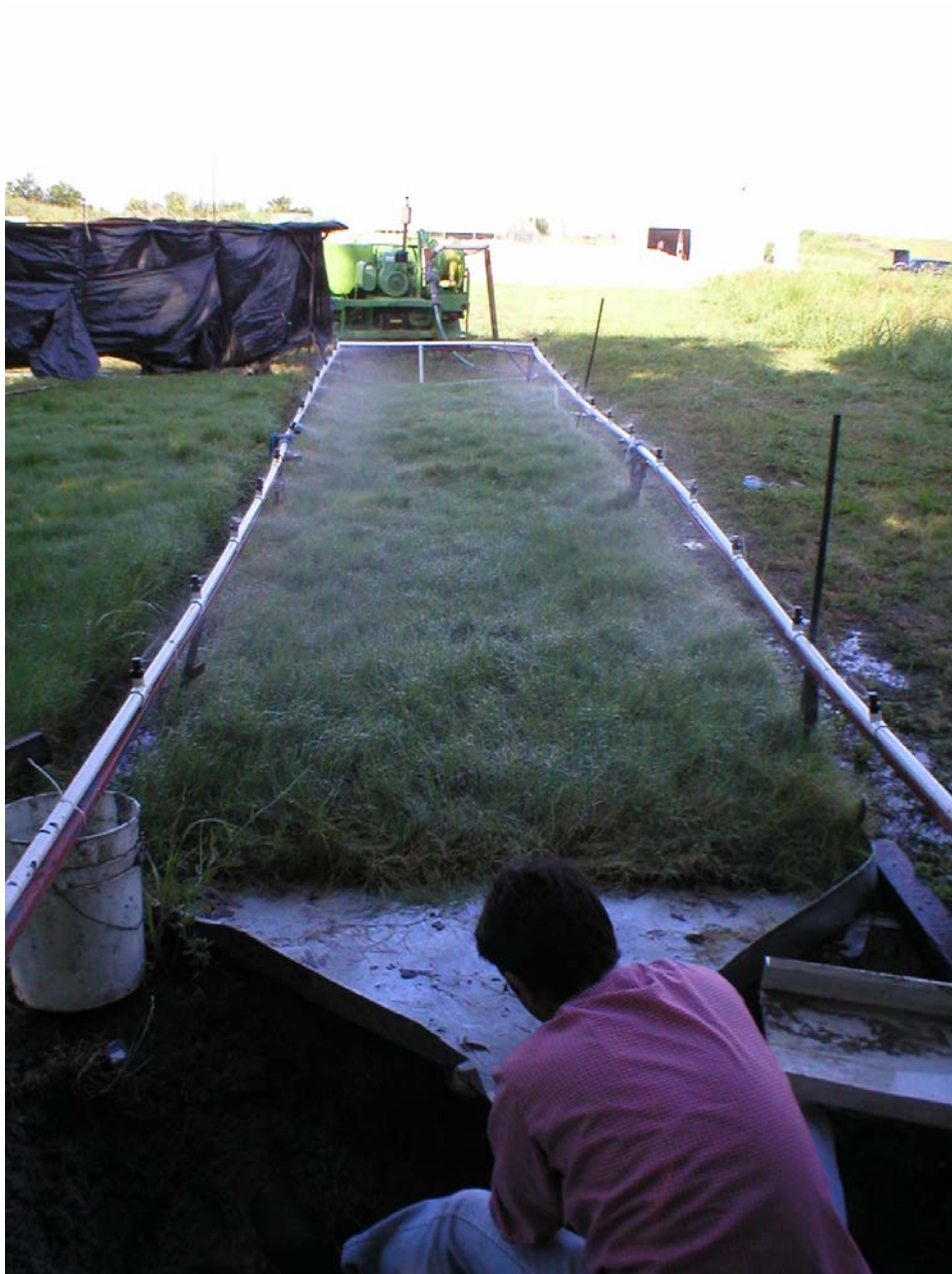
Figure 2 Simulated Rainfall Test
