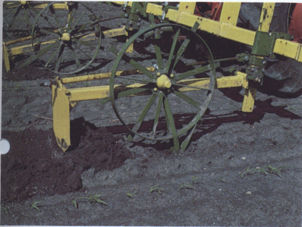
The raising shovel diker features a shovel or disk on the end of a lever arm that is raised and lowered at regular intervals by a step on a large-diameter wheel mounted on the lever.
