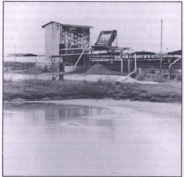
Figure 7. Screening of flushed dairy manure removes fiber that reduces lagoon storage and treatment capacity and reclaims a useful bedding material.
