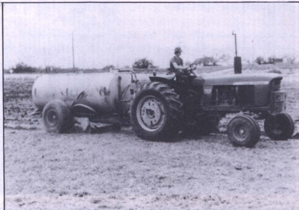
Figure 3. Subsurface injection of liquid manure reduces nitrogen losses, odors, and water pollution potential.
