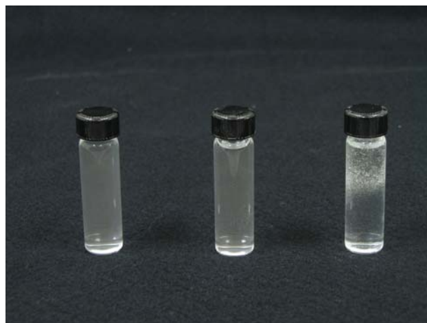
Figure 6.7. Bulk aggregation experiments performed at (L-R) 0.5M NaCl, 0.25M NaCl+0.25M MgSO 4 and, 0.5M MgSO 4 clearly showing aggregation at 0.5M MgSO 4 as predicted.
